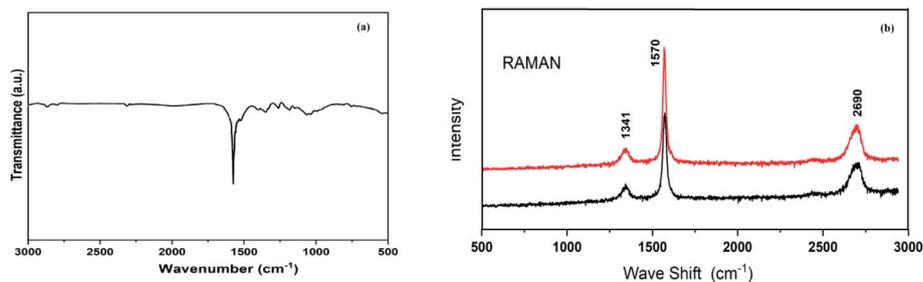
Fig. 2 (a) The FT-IR spectrum of reused graphite and (b) Raman spectra of fresh and reused graphite.
