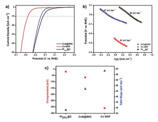
Fig. 11 (a) The HER polarization curves of CoS@SNC, Co MOF, and  $Pt_{20\%}$ @C electrodes at a scan rate of 10 mV s<sup>-1</sup> in 0.1 M KOH solution. (b) The corresponding Tafel slopes for CoS@SNC, Co MOF, and Pt20%@C. (c) A comparison of the potential and Tafel slope values for CoS@SNC, Co MOF, and Pt<sub>20%</sub>@C.
