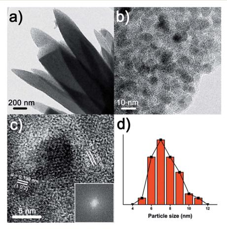
Fig. 2 (a) and (b) TEM and (c) HRTEM images of CoS@SNC (inset of (c): the SAED pattern). (d) The size distribution diagram of CoS particles corresponding to TEM image data.
