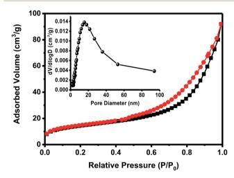
Fig. 5 The  $N_2$  adsorption-desorption isotherm of CoS@SNC (inset: the corresponding pore size distribution).
