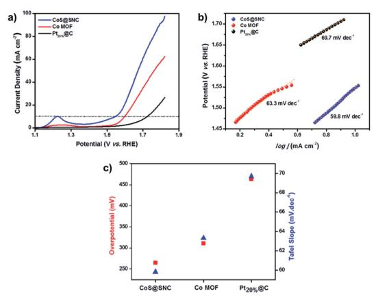
Fig. 9 (a) OER polarization curves of CoS@SNC, Co MOF, and  $Pt_{20\%}$ @C electrodes at a scan rate of 10 mV s<sup>-1</sup> in 0.1 M KOH solution. (b) The corresponding Tafel slopes for CoS@SNC, Co MOF, and  $Pt_{20\%}$ @C. (c) A comparison of the potential and Tafel slope values for CoS@SNC, Co MOF, and  $Pt_{20\%}$ @C.
