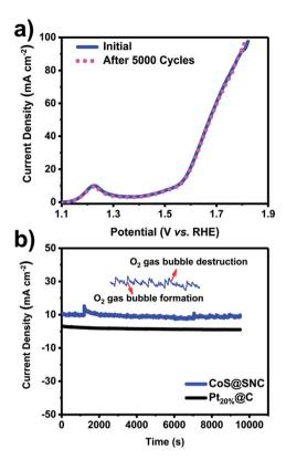
Fig. 10 (a) Polarization curves collected before and after the stability testing of CoS@SNC towards the OER. (b) Chronoamperometric durability testing at 1.54 V.
