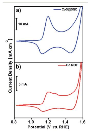
Fig. 7 Cyclic voltammetry plots of (a) CoS@SNC and (b) Co MOF electrodes at a scan rate of  $10~{\rm mV~s}^{-1}$  over the voltage range of  $0.82-1.6~{\rm V}$  vs. RHE in  $0.1~{\rm M}$  KOH.
