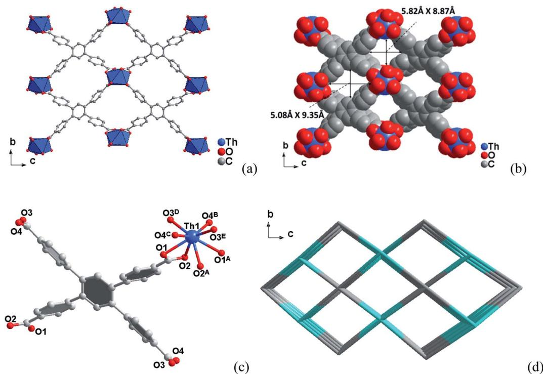
Fig. 1 (a) Three-dimensional framework structure of compound 1 along the  $a$  axis. (b) The corresponding space-filling models with the pore diameters obtained by taking the van der Waals radii. (c) Coordination environments of the Th(IV) sites in compound 1. (d) Topology framework for compound 1 showing the channels along [100] direction.
