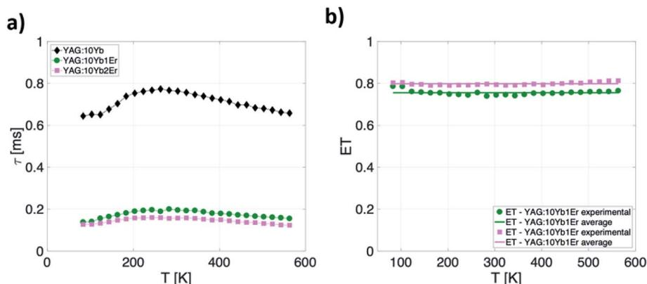
**Fig. 6** (a) Temperature dependence of the  ${}^2\text{F}_{5/2}$  lifetime for YAG:10Yb1Er, YAG:10Yb2Er and YAG:10Yb samples and (b) temperature-dependence of  $\text{Yb}^{3+} \rightarrow \text{Er}^{3+}$  energy transfer.
