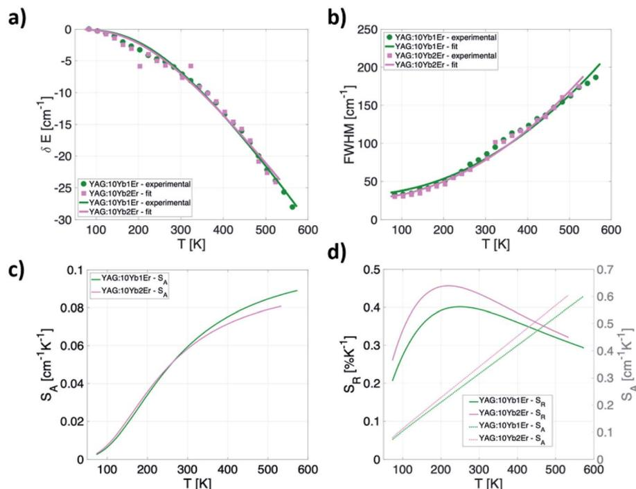
Fig. 5 Temperature dependences of (a) band shift; (b) FWHM; (c) absolute sensitivities obtained via band shift readout; (d)  $S_A$  and  $S_R$  obtained via FWHM readout for YAG:10Yb1Er and YAG:10Yb2Er samples.
