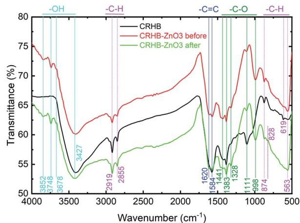
Fig. 9 FTIR of CRHB and CRHB-ZnO<sub>3</sub> before and after the adsorption of heavy metals.
