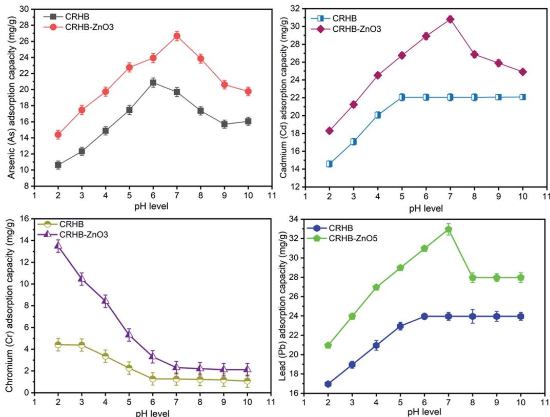
Fig. 2 Effect of initial solution pH on heavy metals adsorption by CRHB and CRHB-ZnO<sub>3</sub>.
