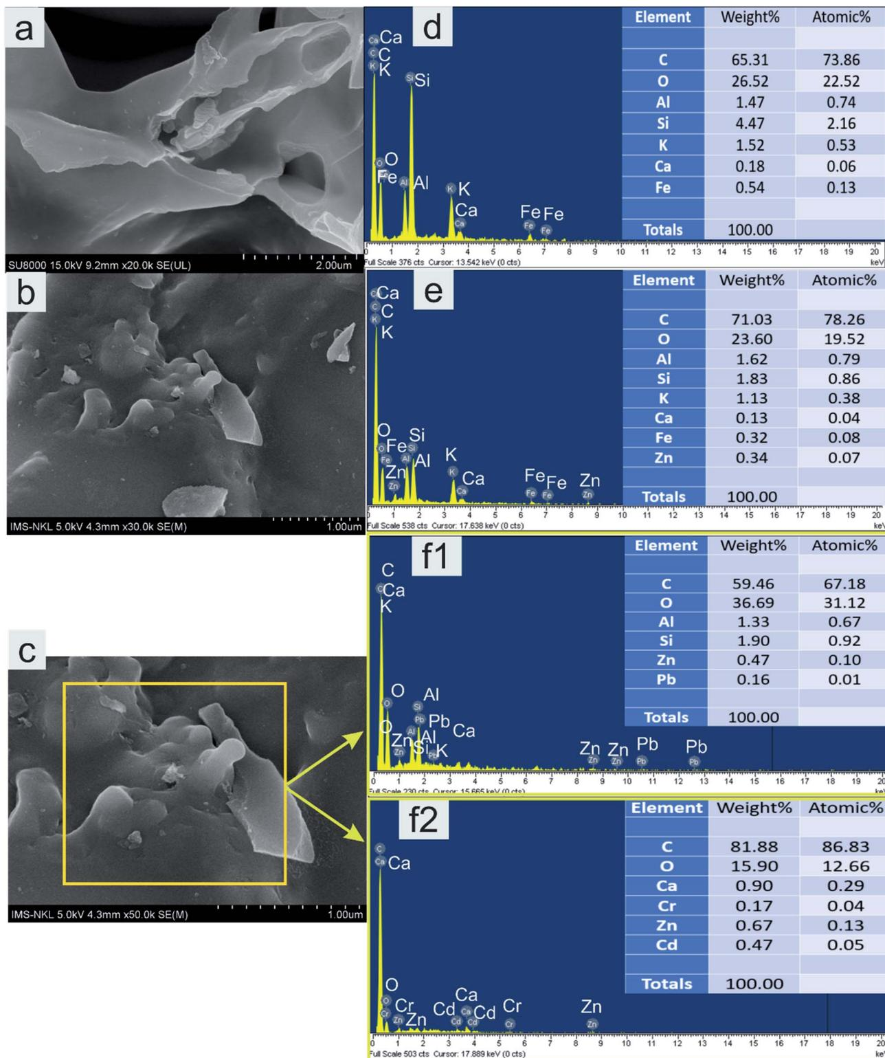
Fig. 7 SEM images and EDS profiles of CRHB (a and d) and CRHB-ZnO<sub>3</sub> (b and e) before and after adsorption (c, f1 and f2).
