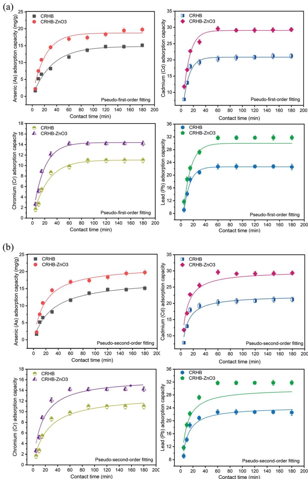
Fig. 3 (a) Pseudo-first-order model of As(III), Cd(II), Pb(II), and Cr(VI) adsorption onto CRHB and CRHB-ZnO<sub>3</sub>. (b) Pseudo-second-order model of As(III), Cd(II), Pb(II), and Cr(VI) adsorption onto CRHB and CRHB-ZnO<sub>3</sub>.
