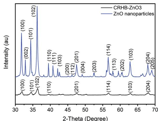
Fig. 5 Graph of XRD ZnO nanoparticles and CRHB-ZnO3.
