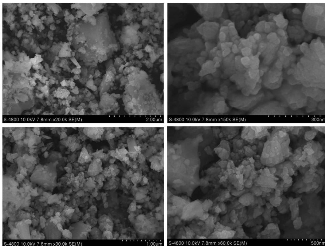
Fig. 6 Field emission scanning electron microscopy (FESEM) images of ZnO nanoparticles.
