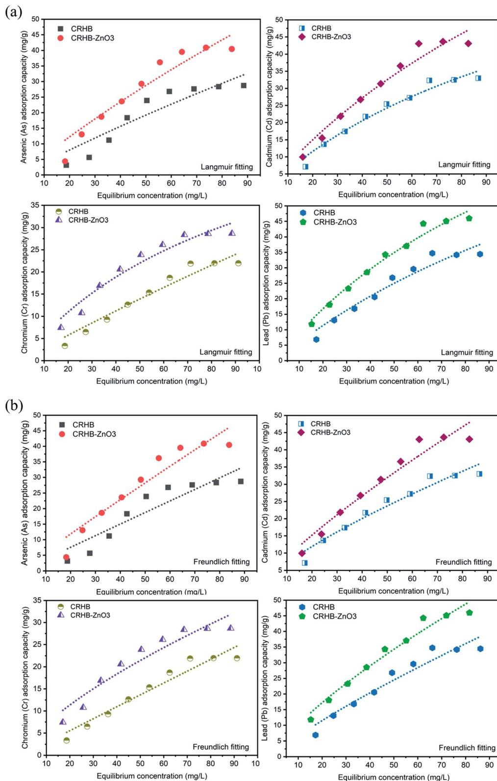
Fig. 4 (a) Langmuir isotherm of heavy metals adsorption onto CRHB and CRHB-ZnO<sub>3</sub>. (b) Freundlich isotherm of heavy metals adsorption onto CRHB and CRHB-ZnO<sub>3</sub>.
