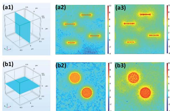
Fig. 11 (a1) Perpendicular cross-section model, and (a2) space charge density in two-dimensional model of MgAl LDH/PVDF and (a3) Ni-MgAl LDH/PVDF nanocomposites. (b1) Parallel cross-section model, and (b2) space charge density in two-dimensional model of MgAl LDH/PVDF and (b3) Ni-MgAl LDH/PVDF nanocomposite.
