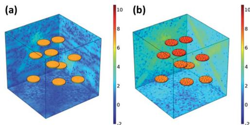
Fig. 10 Space charge density in three-dimensional model of (a) MgAl LDH/PVDF and (b) Ni-MgAl LDH/PVDF nanocomposites.
