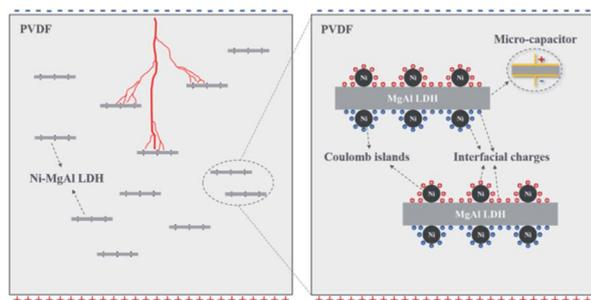
Fig. 5 Schematic diagram of multiple functions of Ni-MgAl LDH nanosheets in nanocomposites.
