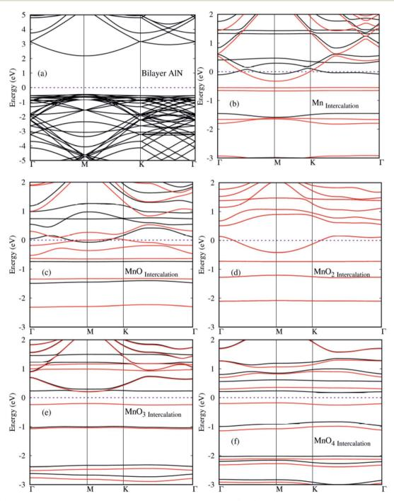
Fig. 5 (a)–(f) Spin polarized electronic structures for  $MnO_x$  cluster-intercalated BL/AlN (4  $\times$  3) supercell structures. Black and Red lines depict spin up and spin down bands, respectively.
