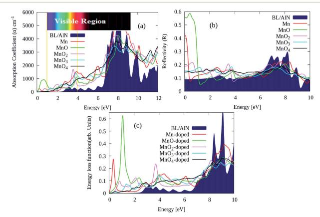
Fig. 7 (a) Absorption coefficient ' $\alpha'$ , (b) reflectivity 'R' and (c) ELS parameters of pure and MnO<sub>x</sub> clusters intercalated BL/AlN systems, respectively.
