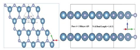
Fig. 1 Illustration for atomic structure of 4 × 3 BL/AIN system (a) normal and (b) in-plane view of optimized geometry of BL/AIN system.
