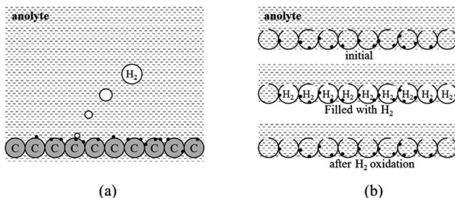
Fig. 4 Hydrogen release during borohydride electrooxidation on an anode supported with solid carbon (a) and porous carbon (b). This figure has been adapted from ref. 55 with permission from WILEY-VCH, copyright 2015.
