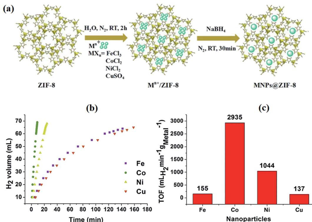
Fig. 13 Synthesis scheme of metal/ZIF-8 nanocatalysts (a), hydrogen release rate from  $\text{NaBH}_4$  hydrolysis for various metal NPs (b), comparison of turnover frequency (TOF) values (c). This figure has been adapted from ref. 130 with permission from WILEY-VCH, copyright 2019.
