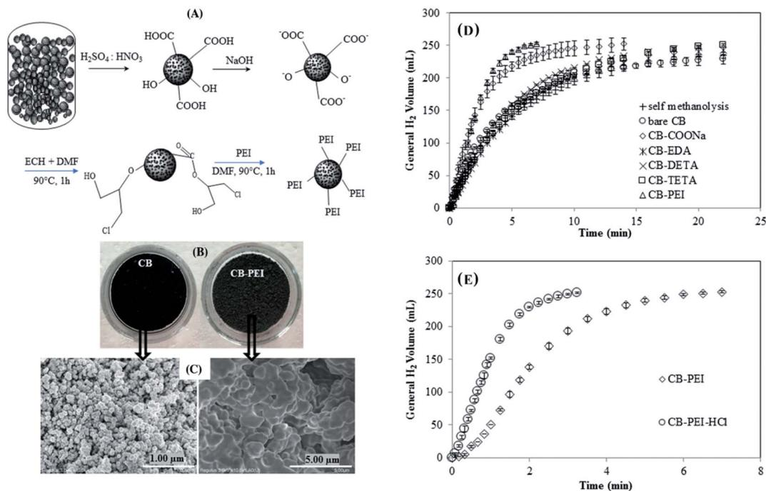
Fig. 8 The process of car tire rubber (CB) modification with PEI (A); images from a digital camera and scanning electron microscopy (B and C); hydrogen release rate from NaBH<sub>4</sub> alcoholysis of unmodified and modified carbons (D and E). This figure has been adapted from ref. 84 with permission from WILEY-VCH, copyright 2019.
