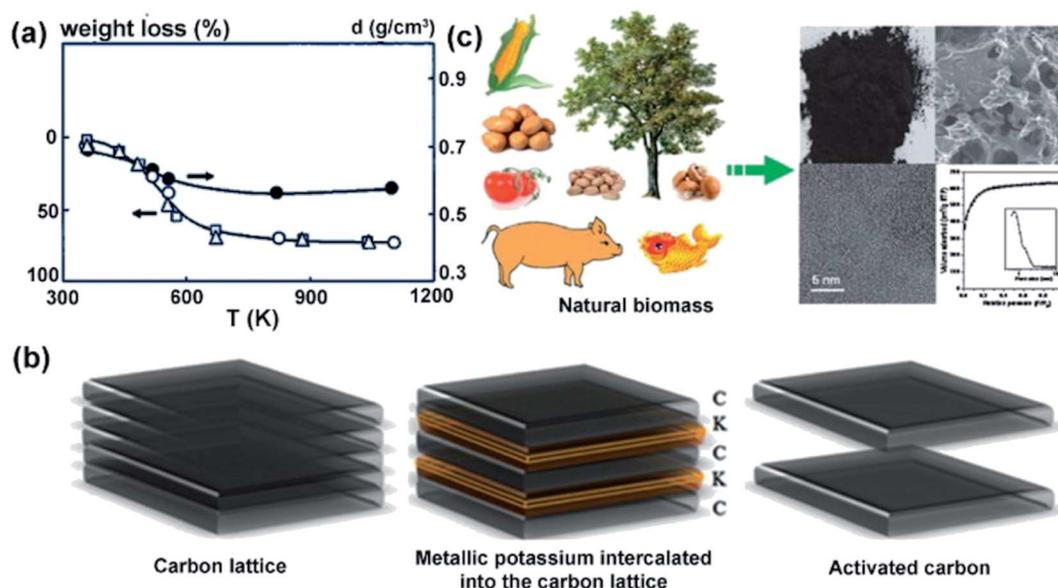
Fig. 7 Change in weight loss for ( $\Delta$ ) almond shells, ( $\square$ ) olive stones and ( $\circ$ ) peach stones during pyrolysis (a); activation mechanism using KOH as activating agent (b); biomass as a source of ACs (c). This figure has been adapted from ref. 67 with permission from TAYLOR & FRANCIS, copyright 2017.
