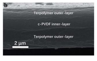
Fig. 2 (a) <sup>1</sup>H NMR spectra of PVDF, unsaturated and terpolymer PVDF-based polymers. (b) Cross-section SEM image of tri-layered composite film with 30 vol% of c-PVDF.
