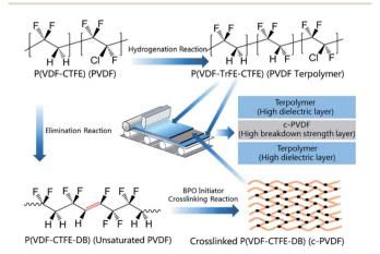
Fig. 1 Molecules of P(VDF-CTFE), P(VDF-CTFE-DB), P(VDF-TrFE-CTFE) and procedures for fabricating the tri-layered composite films.
