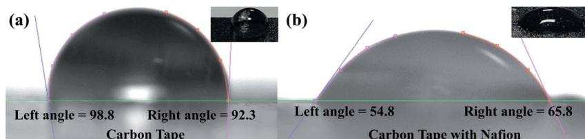
Fig. 2 Image of a sessile water drop on (a) an untreated carbon tape and on (b) an Nf coated carbon tape captured using a goniometer. The water contact angles are mentioned in the figures. Inset at the top right corner of each figure shows photographs of the same.
