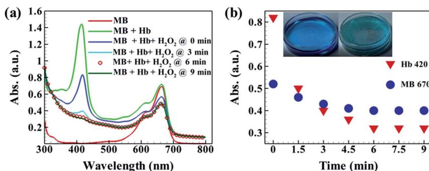
Fig. 9 Plot (a) shows UV-Vis spectroscopy of MB, MB with Hb, and solution of MB, Hb, and  $\text{H}_2\text{O}_2$  together at time intervals 0, 3, 6, 9 min, respectively. Plot (b) shows UV-Vis degradation kinetics, in terms of peak absorption, of MB, and Hb in presence of  $\text{H}_2\text{O}_2$  which is undergoing bio-Fenton reaction. Left and right inset in plot (b) shows color of MB before ( $t = 0$ ) and after ( $t = 9 \text{ min}$ ) degradation.
