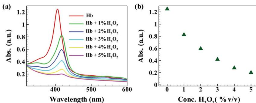
Fig. 8 Plot (a) shows UV-Vis spectroscopy of Hb, Hb in 1%  $\text{H}_2\text{O}_2$ , Hb in 2%  $\text{H}_2\text{O}_2$ , Hb in 3%  $\text{H}_2\text{O}_2$ , Hb in 4%  $\text{H}_2\text{O}_2$ , and Hb in 5%  $\text{H}_2\text{O}_2$ , respectively. Plot (b) shows maximum absorption in UV-Vis spectroscopy at wavelength  $\sim 420$  nm against (v/v)% concentration of  $\text{H}_2\text{O}_2$ , in terms of peak absorption.
