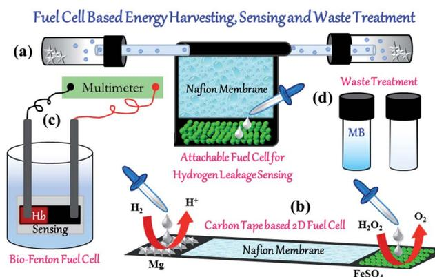
Fig. 1 (a) Schematics of carbon tape-based PEM fuel cell, where  $\text{H}_2$  is generated inside vials and fed to the PEM membrane through connecting pipes. (b) Depicts PEM fuel cell on carbon tape with proximate open sources of  $\text{H}_2$  and  $\text{O}_2$ . (c) Represents prototype of BF fuel cell. (d) Shows MB dye degradation in the presence of Bio Fenton's reaction.
