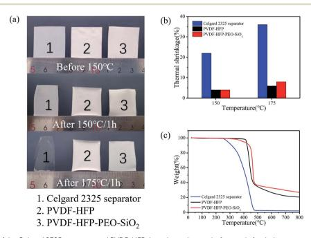
Fig. 2 (a) Photographs of the Celgard 2325 separator and PVDF-HFP-based membranes before and after being exposed to 150 °C and 175 °C for 1 h. (b) Thermal shrinkage of membranes after heat-treatment. (c) TG curves for various membranes.
