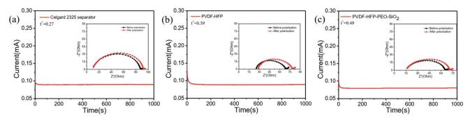
Fig. 5 Chronoamperometry curves of (a) Celgard 2325 separator, (b) PVDF-HFP, (c) PVDF-HFP-PEO-SiO<sub>2</sub> in the symmetrical Li/GPE/Li cells. AC impedances before and after polarization are shown in the inset.
