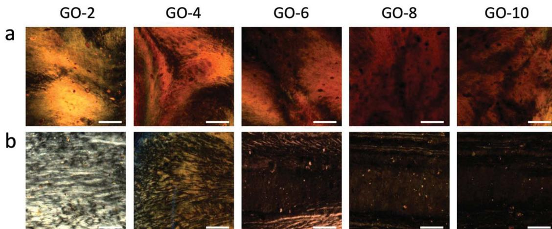
Fig. 4 Polarized optical microscope (POM) images of (a) GO dispersions prepared by drop dispensing and (b) GO dispersions prepared by extrusion from the coat-hanger die. Scale bar represents 200  $\mu\text{m}$ .
