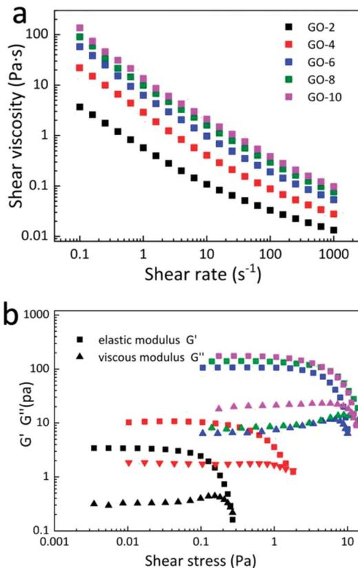
Fig. 1 Rheological behaviour of GO aqueous dispersions. (a) The flow curves show viscosity rapidly increases as GO dispersions concentrations raises from 2  $\text{mg mL}^{-1}$  to 10  $\text{mg mL}^{-1}$ , and viscosity of all 5 different GO dispersion concentrations decreases as shear rate increases. (b) Different elastic modulus ( $G'$ ) and viscous modulus ( $G''$ ) of 5 GO dispersions.
