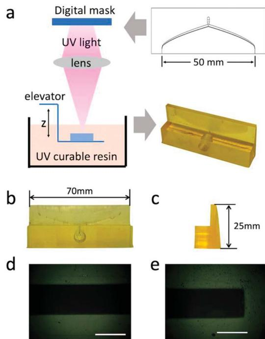
**Fig. 3** (a) Schematic diagram of the fabrication process of the coat-hanger die by photo-curing 3D printer, the outlet length is 50 mm. (b) and (c) are front view and side view of coat-hanger die, respectively. The length and height are 70 mm and 25 mm. (d) and (e) are the optical microscope photos of the center and edge of the die's outlet. Scale bar represents 100  $\mu\text{m}$ .
