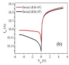
Fig. 4 Diode ( $I_{ds}-V_{ds}$ ) characteristics curves of p-WSe<sub>2</sub>/n-WS<sub>2</sub> heterojunction at  $V_{bg}=-40$  V. (a) Linear scale (b) semi-log scale.
