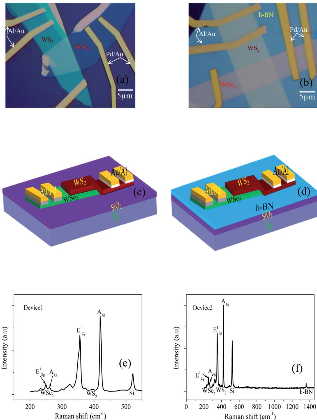
**Fig. 1** (a) and (b) An optical microscopic image of the p-WSe<sub>2</sub>/n-WS<sub>2</sub> heterojunction diode of device1 and device2 respectively. (c) and (d) Schematic device geometry of device1 and device2, respectively. (e) and (f) Raman spectra of device1 and device2 at the junction with laser excitation wavelength of 514 nm.
