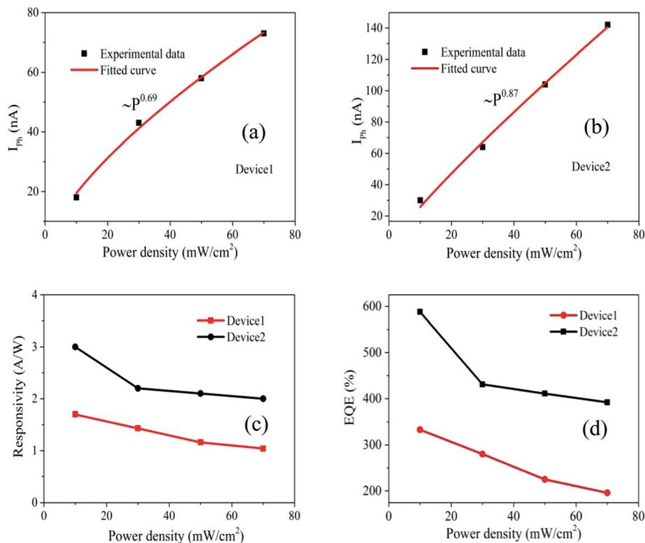
Fig. 6 (a) and (b) Self-driven photocurrent ( $I_{ph}$ ) vs. incident photo-power density on device1 and device2 respectively, where red curves show the power-law fitting. (c) and (d) Responsivity and EQE as a function of power density, respectively.
