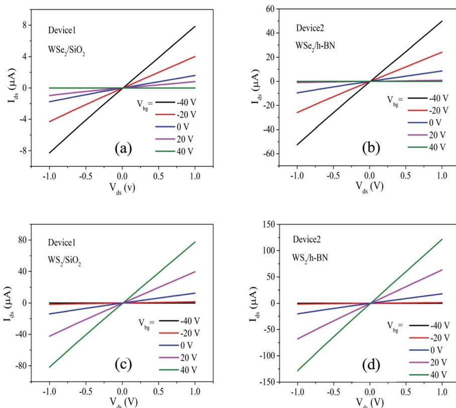
Fig. 3 Linear  $I_{ds}$ - $V_{ds}$  characteristics curve of TMDs at different  $V_{bg}$  on different substrates. (a) and (b) FL-WSe<sub>2</sub> on SiO<sub>2</sub> and h-BN substrates respectively. (c) and (d) FL-WS<sub>2</sub> on SiO<sub>2</sub> and h-BN substrates respectively.
