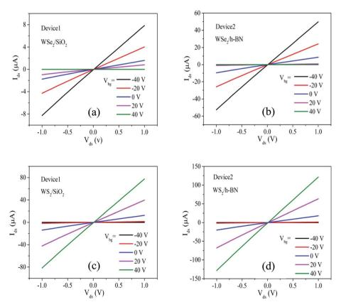
Fig. 3 Linear  $I_{\rm ds}$  –  $V_{\rm ds}$  characteristics curve of TMDs at different  $V_{\rm bg}$  on different substrates. (a) and (b) FL-WSe<sub>2</sub> on SiO<sub>2</sub> and h-BN substrates respectively. (c) and (d) FL-WSe<sub>2</sub> on SiO<sub>2</sub> and h-BN substrates respectively.
