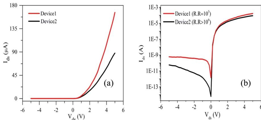
Fig. 4 Diode ( $I_{ds}$ - $V_{ds}$ ) characteristics curves of p-WSe<sub>2</sub>/n-WS<sub>2</sub> heterojunction at  $V_{bg} = -40$  V. (a) Linear scale (b) semi-log scale.
