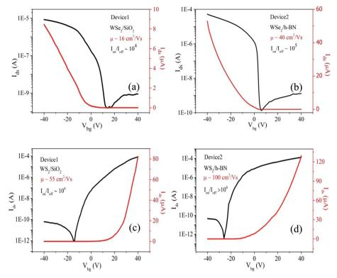
Fig. 2 Transfer characteristics curve ( $I_{ds}-V_{bg}$ ) of each FL flake on different substrates at  $V_{ds}=1$  V. (a) and (b) FL-WSe<sub>2</sub> showing p-type characteristic on SiO<sub>2</sub> and h-BN substrates respectively. (c) and (d) FL-WS<sub>2</sub> showing n-type characteristic on SiO<sub>2</sub> and h-BN substrate respectively.
