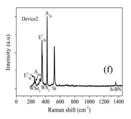
Fig. 1 (a) and (b) An optical microscopic image of the p-WSe $_2$ /n-WS $_2$  heterojunction diode of device1 and device2 respectively. (c) and (d) Schematic device geometry of device1 and device2, respectively. (e) and (f) Raman spectra of device1 and device2 at the junction with laser excitation wavelength of 514 nm.
