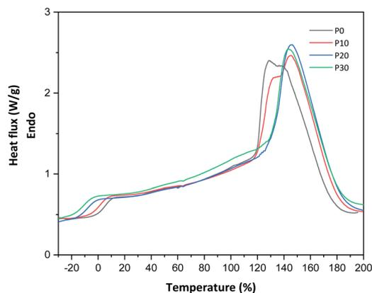
Fig. 4 DSC curves of developed PFJ films.
