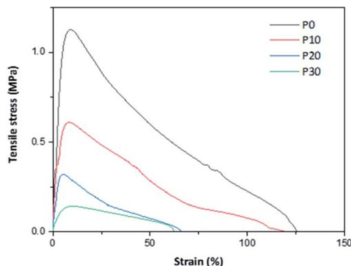
Fig. 6 Examples of tensile stress–strain curves of the PFJ films.
