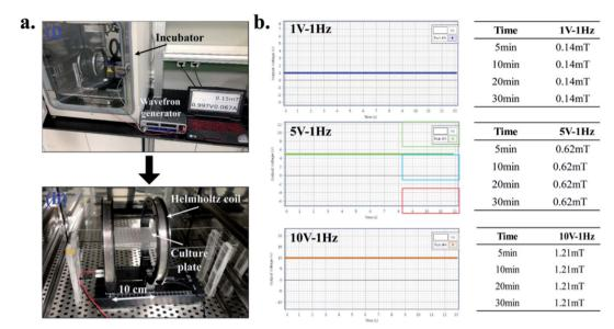
Fig. 1 The EMF device setup. (a) Installation of EMF device with Helmholtz coils, placed inside the incubator (i and ii), and (b) the different EMFs exposure conditions with corresponding magnetic field intensity used in this study.
