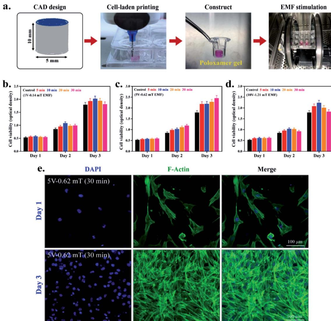
Fig. 5 (a) Schematic illustration of cell printing using P407 and EMFs stimulation. Cytotoxicity evaluation of cell-laden 3D constructs in (b) 1 V–0.14 mT EMF, (c) 5 V–0.62 mT EMF, and (d) 10 V–1.21 mT EMF by WST-1 assay at indicated time intervals. (e) Representative fluorescence microscopy images of EMFs-stimulated SCAPs at indicated time intervals (scale bar: 100  $\mu$ m). Data are mean  $\pm$  SD of triplicated experiments, statistical significance at \* $p$  < 0.05.
