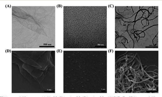
Fig. 1 The TEM images of different material: (A) rGO, (B) hemin-rGO, (C) hemin-rGO-cMWCNTs. The SEM images of different material: (D) rGO. (E) hemin-rGO. (F) hemin-rGO-cMWCNTs.
