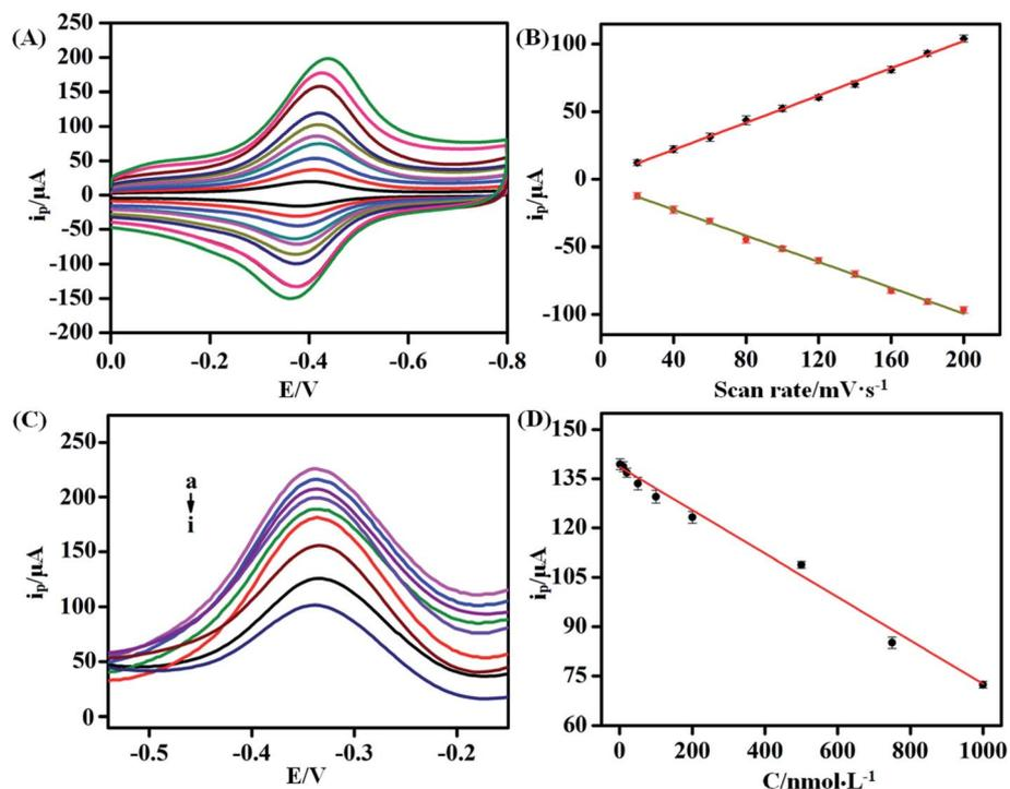
Fig. 6 (A) The CV plots of KANA/aptamer/rGO-hemin-cMWCNTs/GCE at different scan rates (20, 40, 60, 80, 100, 120, 140, 160, 180, 200  $\text{mV s}^{-1}$ ) in 0.1 M PBS (pH 6.0). (B) The relationship between peak current and scan rates. (C) The DPV plots of KANA/aptamer/hemin-rGO-cMWCNTs/GCE modified with different concentrations of KANA (a to i: (1 nM, 10 nM, 20 nM, 50 nM, 100 nM, 200 nM, 500 nM, 750 nM, 1000 nM)). (D) The relationship between peak current and the concentration of KANA.
