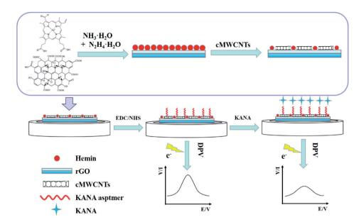
Scheme 1 The schematic diagram of the construction of the KANA/aptamer/hemin-rGO-cMWCNTs/GCE for the detection of KANA.
