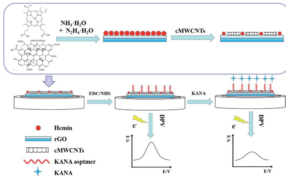
Scheme 1 The schematic diagram of the construction of the KANA/apptamer/hemin-rGO-cMWCNTs/GCE for the detection of KANA.
