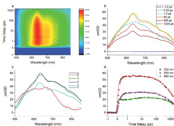
**Fig. 4** Results of transient absorption spectroscopy (TAS) studies of **FO52** solution. (a) A 2D color map of the TAS results; (b) TAS at various delay times; (c) spectral components extracted from global and target analysis, providing information about the evolution of TAS; and (d) kinetic traces with numerical fitting at various wavelengths.
