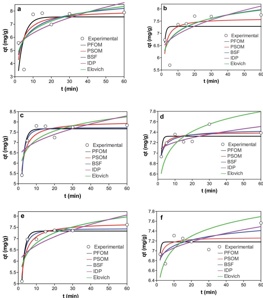
Fig. 8 Graphs showing the adsorption kinetics of (a) KCB (b) KCB-A (c) KCB-B on CIP (d) KCB (e) KCB-A and (f) KCB-B on TET.
