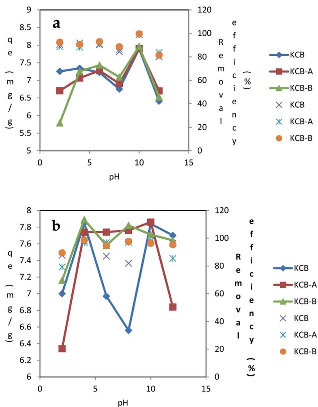
Fig. 5 Effect of pH on the adsorption of (a) TET (b) CIP using KCB, KCB-A and KCB-B (initial concentration =  $40 \text{ mg L}^{-1}$ ; contact time = 60 minutes; adsorbent dosage =  $0.05 \text{ g}$ ; temperature =  $303 \text{ K}$ ).
