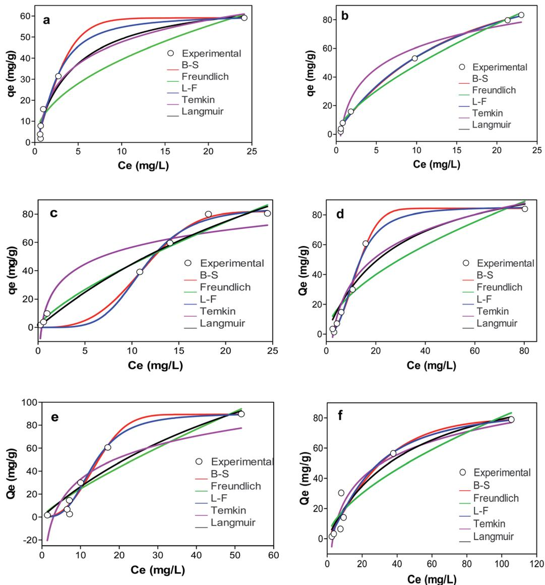
Fig. 6 Graphs showing the adsorption isotherms of (a) KCB (b) KCB-A (c) KCB-B on CIP (d) KCB (e) KCB-A and (f) KCB-B on TET.
