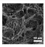
Fig. 9 High-magnification SEM image of the coating layers formed by N-50 (5 mL, 10 mg mL $^{-1}$ ) with 2  $\mu$ L water.
