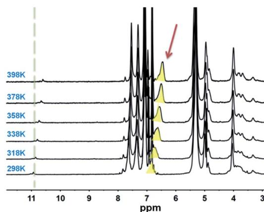
Fig. 5 Variable temperature <sup>1</sup>H NMR spectra of N-45 in 1,2-dichlorobenzene-d<sup>4</sup>.
