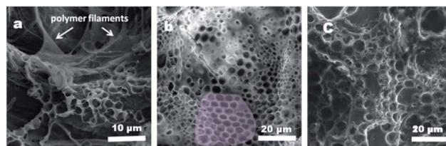
Fig. 2 SEM images of PBTF-30 micro-patterns formed at different concentrations: (a) 5 mg mL<sup>-1</sup>; (b) 15 mg mL<sup>-1</sup>; (c) 30 mg mL<sup>-1</sup>.
