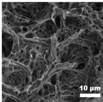
Fig. 9 High-magnification SEM image of the coating layers formed by N-50 (5 mL, 10 mg mL<sup>-1</sup>) with 2  $\mu$ L water.
