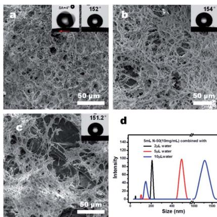
Fig. 8 SEM images of the coating layers formed by N-50 (5 mL, 10 mg mL<sup>-1</sup>) with different water contents, 2  $\mu$ L (a), 5  $\mu$ L (b), and 10  $\mu$ L (c) and the DLS curves of the corresponding nano-emulsions (d).
