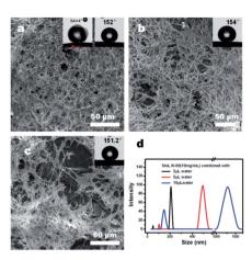
Fig. 8 SEM images of the coating layers formed by N-50 (5 mL, 10 mg mL $^{-1}$ ) with different water contents, 2  $\mu$ L (a), 5  $\mu$ L (b), and 10  $\mu$ L (c) and the DLS curves of the corresponding nano-emulsions (d).
