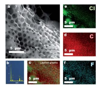
Fig. 4 Enlarged SEM images (a) and EDS mapping images (b-f) of honeycomb coating layers prepared by PBTF-50.
