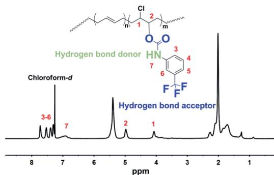
Fig. 1 <sup>1</sup>H NMR spectra of PBTF-30 in chloroform-d.
