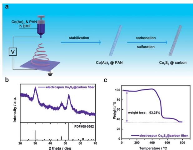
Fig. 1 (a) Schematic of synthesis electrospun Co<sub>9</sub>S<sub>8</sub>@carbon fiber; (b) the XRD pattern of Co<sub>9</sub>S<sub>8</sub>@carbon fiber; (c) the TGA curve of Co<sub>9</sub>S<sub>8</sub>@carbon fiber.
