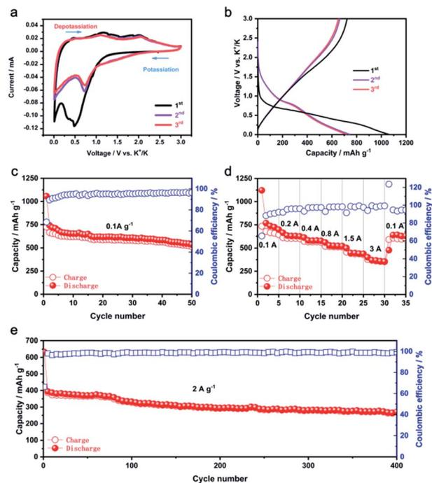
Fig. 3 (a) Cyclic voltammograms (CV) curve at a scanning rate of  $0.1 \text{ mV s}^{-1}$ ; (b) galvanostatic discharge/charge potential profiles of the first three cycles at  $0.1 \text{ A g}^{-1}$ ; (c) cycling performance at  $0.1 \text{ A g}^{-1}$ ; (d) rate performance at different current densities from 0.1 to  $3 \text{ A g}^{-1}$  and (e) long-term cycling performance at  $2 \text{ A g}^{-1}$  of  $\text{Co}_9\text{S}_8$ @carbon fiber electrode.
