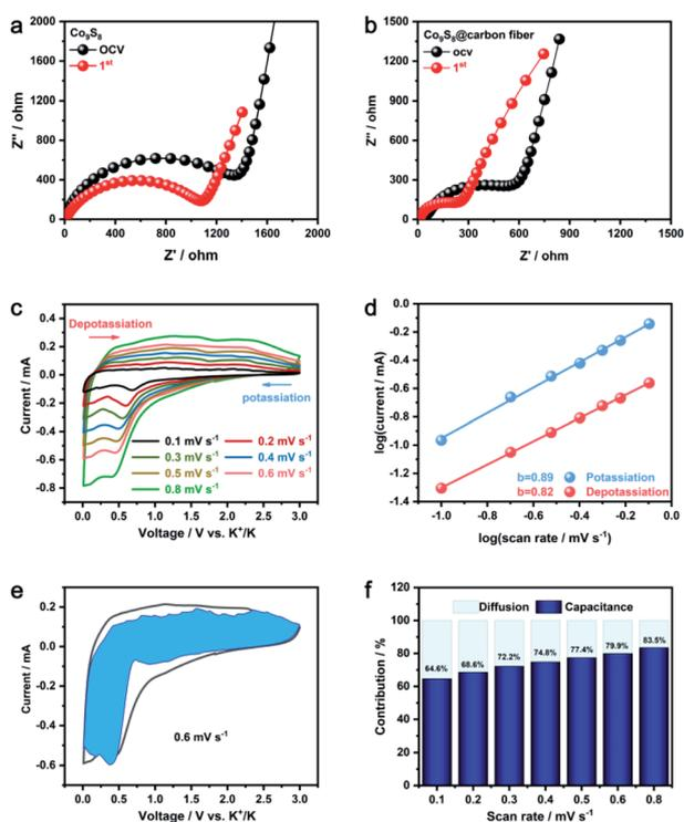
Fig. 4 Nyquist plots of OCV and after first cycle of (a)  $\text{Co}_9\text{S}_8$  electrodes; (b) electrospun  $\text{Co}_9\text{S}_8$ @carbon fiber electrodes; (c) CV curves of the  $\text{Co}_9\text{S}_8$  electrode at various scan rates; (d)  $\log(i)$  versus  $\log(\nu)$  plots; (e) CV curve with capacitive- and diffusion-controlled contributions at  $0.6 \text{ mV s}^{-1}$ ; (f) the ratio of pseudocapacitive contribution at different scan rates.
