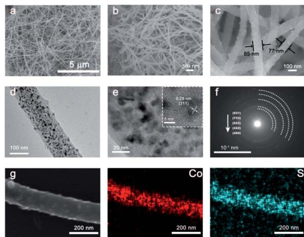
Fig. 2 (a–c) SEM images (d and e) TEM images, (f) selected area electron diffraction (SAED) pattern, (g) element mapping of the as-synthesized  $\text{Co}_9\text{S}_8$ @carbon fiber. The inset of (d) shows the HRTEM image.
