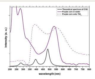
Fig. 3 Experimental absorption spectra of the dye obtained from *Zea mays* in solution and adhered to TiO<sub>2</sub> compared with the theoretical spectrum obtained for C3G.
