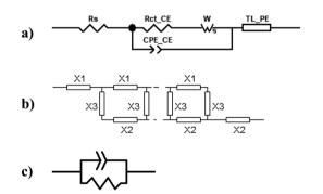
Fig. 15 (a) Equivalent circuit used to adjust the impedance spectra of the manufactured DSSCs. The transmission line TL\_PE follows the scheme shown in (b), where each element  $X_1$ ,  $X_2$  and  $X_3$  becomes a resistor and a phase element in parallel, as shown in (c).
