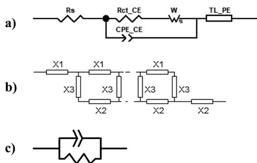
Fig. 15 (a) Equivalent circuit used to adjust the impedance spectra of the manufactured DSSCs. The transmission line TL<sub>PE</sub> follows the scheme shown in (b), where each element X<sub>1</sub>, X<sub>2</sub> and X<sub>3</sub> becomes a resistor and a phase element in parallel, as shown in (c).
