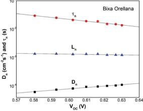
**Fig. 14** Diffusion length of the solar cell calculated from the electron lifetime and the chemical diffusion coefficient.
