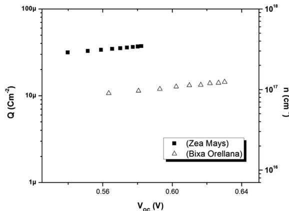
Fig. 8 Extracted charge and electron density obtained as a function of the open circuit voltage in the cells manufactured with *Zea mays* and *Bixa orellana*.
