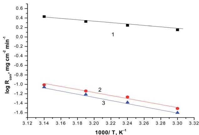
**Fig. 7** The correlation between the  $R_{\text{corr.}}$  and  $1/T$  of SABIC iron in 0.5 M H<sub>2</sub>SO<sub>4</sub> solution devoid of and containing 250 mg l<sup>-1</sup> of VB1 and VB2. (1) 0.5 M H<sub>2</sub>SO<sub>4</sub>, (2) VB1 and (3) VB2.
