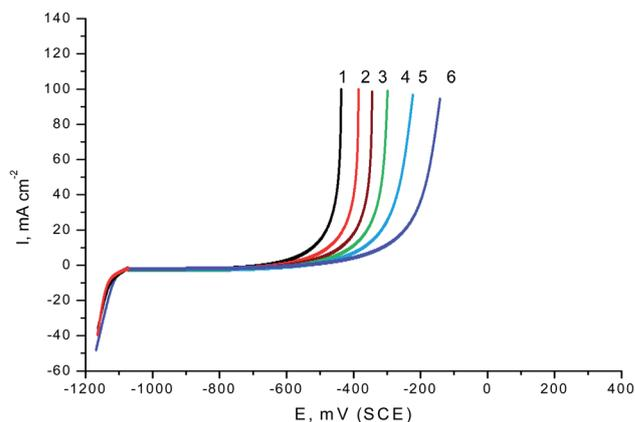
Fig. 2 PDAP curves of SABIC iron in 0.5 M  $H_2SO_4$  including 0.5 M NaCl solutions including various concentrations of VB2 at scan rate 1 mV s. (1) 0.00 mg  $l^{-1}$ , (2) 50 mg  $l^{-1}$ , (3) 100 mg  $l^{-1}$ , (4) 150 mg  $l^{-1}$ , (5) 200 mg  $l^{-1}$  and (6) 250 mg  $l^{-1}$ .
