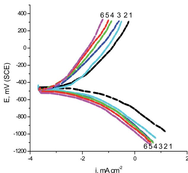
Fig. 1 GP curves of SABIC iron blank 0.5 M H<sub>2</sub>SO<sub>4</sub> solution and contains diverse concentrations of VB2. (1) 0.00 mg l<sup>-1</sup>, (2) 50 mg l<sup>-1</sup>, (3) 100 mg l<sup>-1</sup>, (4) 150 mg l<sup>-1</sup>, (5) 200 mg l<sup>-1</sup> and (6) 250 mg l<sup>-1</sup>.
