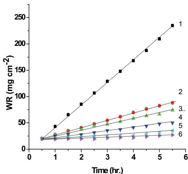
**Fig. 6** WR–time curves of SABIC iron in 0.5 M H<sub>2</sub>SO<sub>4</sub> solution containing some concentrations of VB2 at 303 K. (1) 0.00 mg l<sup>-1</sup>, (2) 50 mg l<sup>-1</sup>, (3) 100 mg l<sup>-1</sup>, (4) 150 mg l<sup>-1</sup>, (5) 200 mg l<sup>-1</sup> and (6) 250 mg l<sup>-1</sup>.
