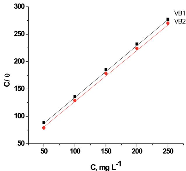
**Fig. 9** Relation between  $CVB/\theta$  versus  $CVB$  for of SABIC iron in blank 0.5 M H<sub>2</sub>SO<sub>4</sub> solution and including some concentrations of VB1 and VB2.
