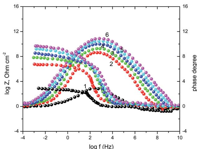
**Fig. 5** Nyquist plots SABIC iron corrosion in the blank 0.5 M H<sub>2</sub>SO<sub>4</sub> and with addition of certain concentrations of VB2. (1) 0.00 mg l<sup>-1</sup>, (2) 50 mg l<sup>-1</sup>, (3) 100 mg l<sup>-1</sup>, (4) 150 mg l<sup>-1</sup>, (5) 200 mg l<sup>-1</sup> and (6) 250 mg l<sup>-1</sup>.
