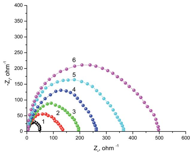
Fig. 4 Nyquist plots SABIC iron corrosion in the blank 0.5 M  $\text{H}_2\text{SO}_4$  and with addition of certain concentrations of VB2. (1) 0.00  $\text{mg l}^{-1}$ , (2) 50  $\text{mg l}^{-1}$ , (3) 100  $\text{mg l}^{-1}$ , (4) 150  $\text{mg l}^{-1}$ , (5) 200  $\text{mg l}^{-1}$  and (6) 250  $\text{mg l}^{-1}$ .
