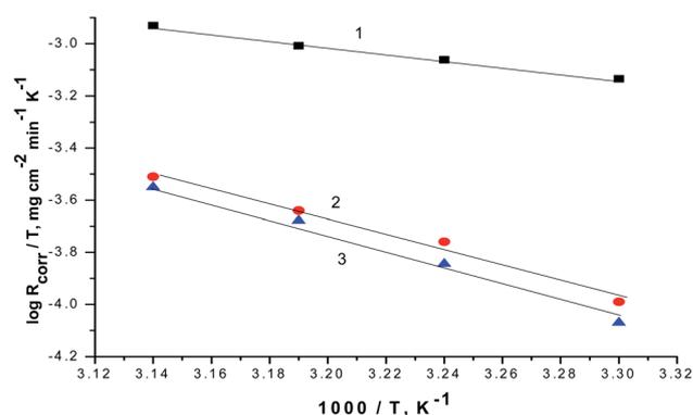
**Fig. 8** The correlation between the  $R_{\text{corr.}}/T$  and  $1/T$  of SABIC iron in 0.5 M H<sub>2</sub>SO<sub>4</sub> solution devoid of and containing 250 mg l<sup>-1</sup> of VB1 and VB2. (1) 0.5 M H<sub>2</sub>SO<sub>4</sub>, (2) VB1 and (3) VB2.
