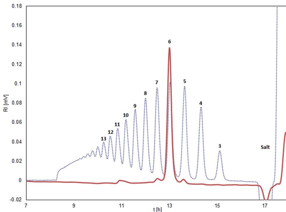
**Fig. 1** Size exclusion chromatogram of chitosan ( $F_A = 0.001$ ) degraded by chitinase from *Streptomyces griseus* (blue dotted line). Isolated chitosan hexamer (red line). The number of glucosamine units in the oligomer peak is given in bold numbers.
