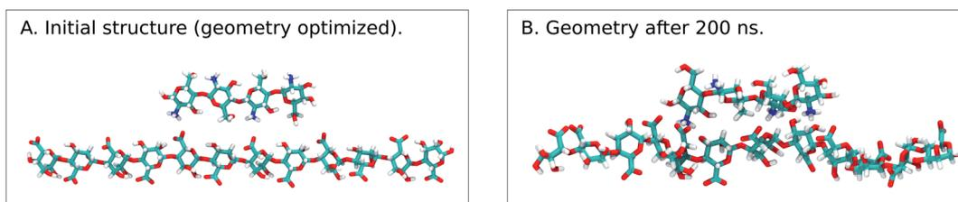
Fig. 6 Snapshots from a MD simulation of the MG-oligomer (DP = 12) and the chitosan oligomer (DP = 4) ( $\text{Na}^+$  and  $\text{Cl}^-$  ions are not shown). (Left) The initial geometry optimized configuration. (Right) The configuration after a MD simulation lasting 200 ns, showing some distortions compared to the initial structure.
