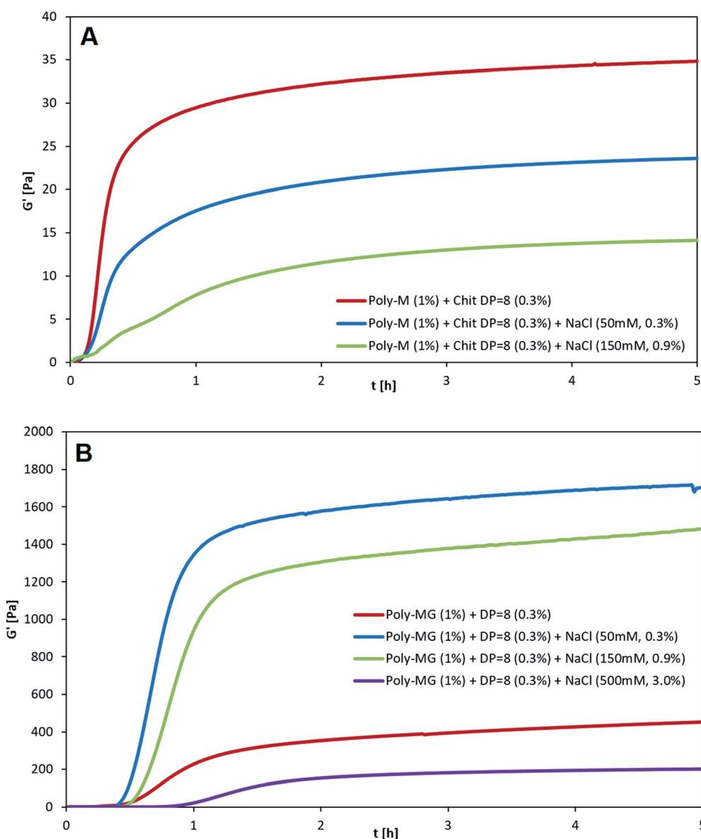
Fig. 4 Influence of NaCl concentration on the kinetics of gelation for (A) poly-M and (B) poly-MG. Alginate concentration at  $10 \text{ g L}^{-1}$  (1%), chitosan octamer concentration at  $3 \text{ g L}^{-1}$  (0.3%), GDL at  $2 \text{ g L}^{-1}$ , NaCl concentration added at 0 mM (red), 50 mM (blue), 150 mM (green), 500 mM (purple).  $G'$  was determined as a function of time.  $G''$  and  $\delta$  are not shown in the figure for reasons of clarity.
