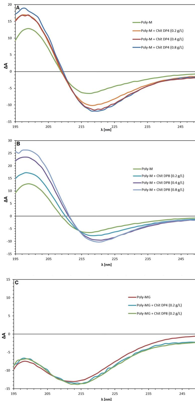
Fig. 5 Circular dichroism spectra of (A) poly-M with chitosan DP = 4; (B) poly-M with chitosan DP = 8; and (C) poly-MG with chitosan DP = 4 and DP = 8. The alginate concentration was consistently at  $0.4 \text{ g L}^{-1}$ . The chitosan concentration ranged from  $0.2$  to  $0.8 \text{ g L}^{-1}$ . All measurements performed at  $\text{pH} = 4.5$  and  $T = 25 \text{ }^\circ\text{C}$ .
