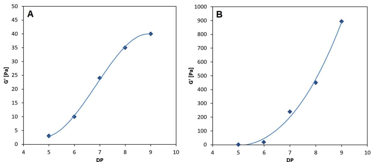
Fig. 3 Final gel strength as a function of degree of polymerization of chitosan. (A) Poly-M; (B) poly-MG. Alginate concentration at  $10 \text{ g L}^{-1}$  (1%). Chitosan concentration at  $3 \text{ g L}^{-1}$  (0.3%). GDL at  $2 \text{ g L}^{-1}$ .  $G'$  value determined after 5 h.
