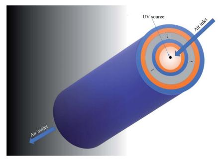
Fig. 2 3D schematic of APCs with an air core and UV source in its center. The structure is proposed to work as part of an air ventilation system where the contaminated air enters one side and comes out as purified air from the pathogens.
