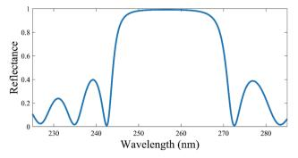
Fig. 3 The reflectance of UV radiation from APC with periodicity number N=20 unit cell that consisted of  $Al_2O_3$  layer with thickness 35 nm and  $SiO_2$  layer with thickness 40 nm.
