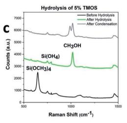
Fig. 1 Synthesis and Raman characterization of CaRGOS formulations. (a and b) Schematic of CaRGOS formulations and encapsulation of hemoglobin for long-term room-temperature storage and (c) complete hydrolysis of 5.0 v/v % tetramethyl orthosilicate (TMOS) was demonstrated by Raman spectra with an elimination of TMOS peak ( $646 \text{ cm}^{-1}$ ) and formation of methanol peak ( $1030 \text{ cm}^{-1}$ ) after a standard microwave synthesis.
