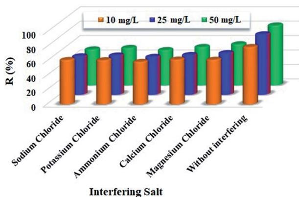
Fig. 6 Effect of interfering species on Cr(VI) ion removal percentage (%R) by the NFe<sub>3</sub>O<sub>4</sub>Starch-Glu-NFe<sub>3</sub>O<sub>4</sub>ED nanocomposite. (Sample volume = 10.0 mL; nanosorbent dose = 10.0 ± 1 mg; Cr(VI) initial concentrations = 10.0, 25.0, and 50.0 mg L<sup>-1</sup>; pH value = 2.0; shaking time = 60.0 min; temperature = 25 °C; mass of interfering salt = 100.0 ± 0.1 mg; shaking speed = 250 rpm).
