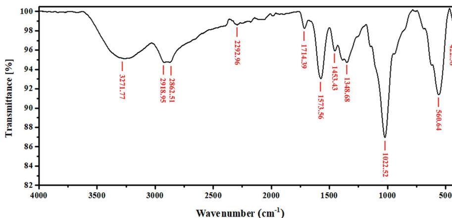
Fig. 1 FT-IR spectrum of the NFe<sub>3</sub>O<sub>4</sub>Starch-Glu-NFe<sub>3</sub>O<sub>4</sub>ED nanocomposite.
