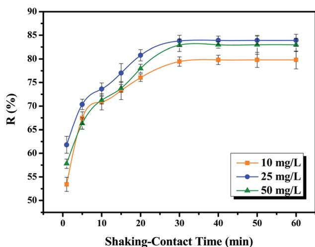
Fig. 4 Effect of contact time on Cr(vi) ion removal percentage (%R) by the  $\text{NFe}_3\text{O}_4\text{Starch-Glu-NFe}_3\text{O}_4\text{ED}$  nanocomposite. (Sample volume = 10.0 mL; nanosorbent dose =  $10.0 \pm 1.0$  mg; Cr(vi) initial concentrations = 10.0, 25.0, and 50.0  $\text{mg L}^{-1}$ ; pH value = 2.0; shaking time = 1.0, 5.0, 10.0, 15.0, 20.0, 30.0, 40.0, 50.0, and 60.0 min; temperature = 25 °C; shaking speed = 250 rpm).
