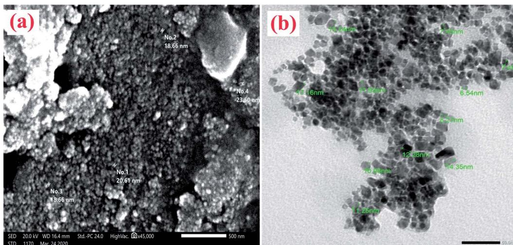
Fig. 2 (a) SEM and (b) HR-TEM images of the NFe<sub>3</sub>O<sub>4</sub>Starch-Glu-NFe<sub>3</sub>O<sub>4</sub>ED nanocomposite.
