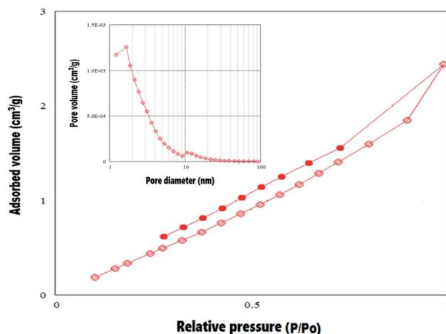
Fig. 3 Nitrogen adsorption-desorption isotherm (inset) pore size of the NFe<sub>3</sub>O<sub>4</sub>Starch-Glu-NFe<sub>3</sub>O<sub>4</sub>ED nanocomposite.
