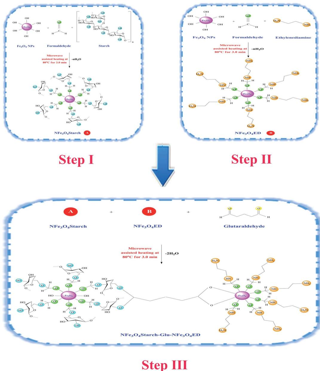
Scheme 1 Synthetic route of the NFe<sub>3</sub>O<sub>4</sub>Starch-Glu-NFe<sub>3</sub>O<sub>4</sub>ED nanocomposite.
