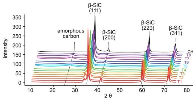
Fig. 5 XRD spectra of samples of the petrified tobacco products (T1–T8, colored) in duplicate and corn husks (CH, black).
