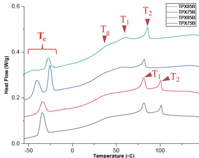
Fig. 2 DSC curves showing first cooling trace of random and block terpolymers with PEG crystallization ( $T_c$ ), glass transition ( $T_g$ ) and LC mesophase transitions ( $T_1$  and  $T_2$ ).  $T_2$  is the LC clearing temperature and generally glass transition temperature and LC mesophase transition of terpolymers lies between 26–37 °C and 80.7–100.9 °C, respectively. A heating/cooling rate of 10 °C min<sup>-1</sup> is used in this study.
