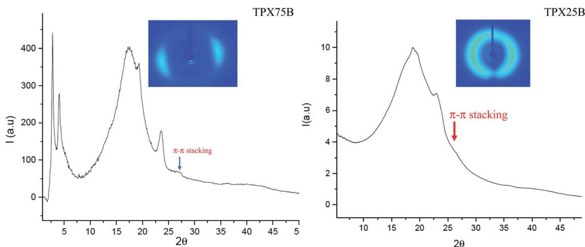
Fig. 3 WAXS pattern obtained from compression molded TPX75B and TPX25B where TPX25B has P(NBCh<sub>9</sub>-b-NBXan-b-NBPEG) with 25/60/15 by composition (wt%). The characteristic peak indicative of face to face  $\pi$ - $\pi$  stacking appears at 0.34 nm. Inset: 2D WAXS pattern of TPX75B and TPX25B confirm preferentially oriented system.
