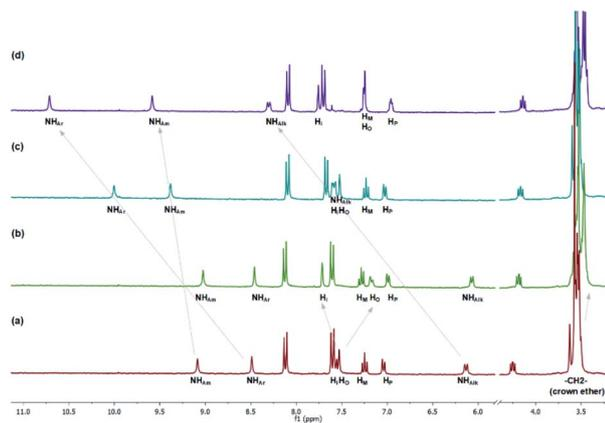
Fig. 2  $^1\text{H}$  NMR spectra: (a) receptor **1**; (b) receptor **1** after addition of 1 eq of  $\text{KPF}_6$ ; (c) receptor **1** after addition of 1 eq of TBA AcO; (d) receptor **1** after addition of 1 eq of  $\text{KPF}_6$  and 1 eq of TBA AcO; (293 K, 3%  $\text{H}_2\text{O}/\text{CD}_3\text{CN}$  solution,  $C_{\text{receptor}} = 3.8 \times 10^{-3}$  M).
