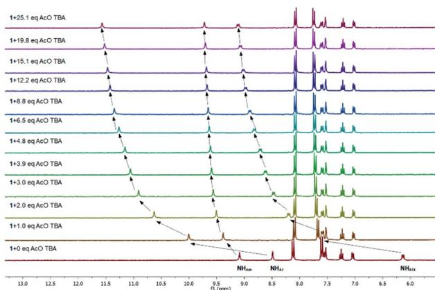
Fig. 3 Partial  $^1\text{H}$  NMR spectra of **1** upon titrant (TBA AcO) addition, (293 K, 3%  $\text{H}_2\text{O}/\text{CD}_3\text{CN}$  solution,  $C_{\text{titrant}} = 1.9 \times 10^{-1}$  M,  $C_{\text{receptor}} = 3.8 \times 10^{-3}$  M).
