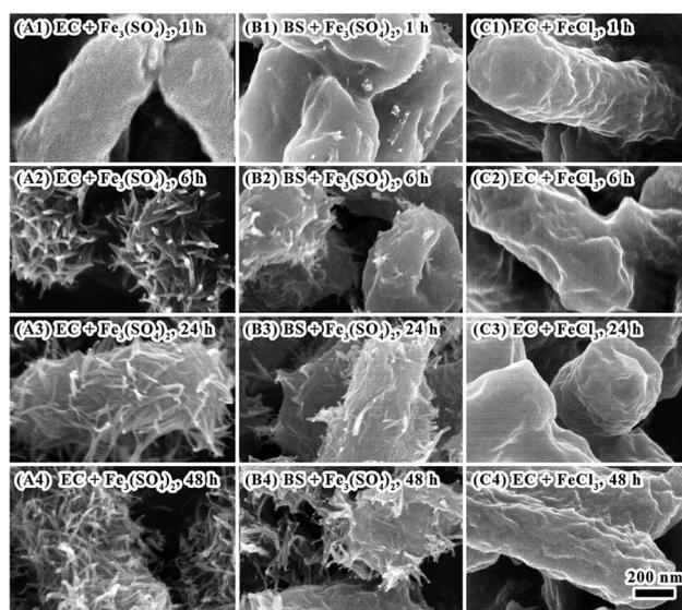
Fig. 4 Panels A1–A4 show oscillating mineralization with  $\text{Fe}_3(\text{SO}_4)_2$  as iron source on *E. coli* for 1, 6, 24 and 48 hours. Panels B1–B4 show oscillating mineralization with  $\text{Fe}_3(\text{SO}_4)_2$  as iron source on *Bacillus subtilis* for 1, 6, 24 and 48 hours. Panels C1–C4 show oscillating mineralization of with  $\text{FeCl}_3$  as iron source on *E. coli* for 1, 6, 24 and 48 hours.
