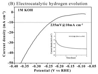
Fig. 7 Panel A shows degradation of methylene blue. Inset of Panel A shows linear relationship between  $\ln(C/C_0)$  and irradiation time. Panel B shows polarization curve of iron biominerals for HER in 1 M KOH with a potential scan rate of 5 mV s<sup>-1</sup>. Inset of Panel B shows durable operation test of iron biominerals electrodes operated at designed  $\eta$  (10 mA cm<sup>-2</sup>).
