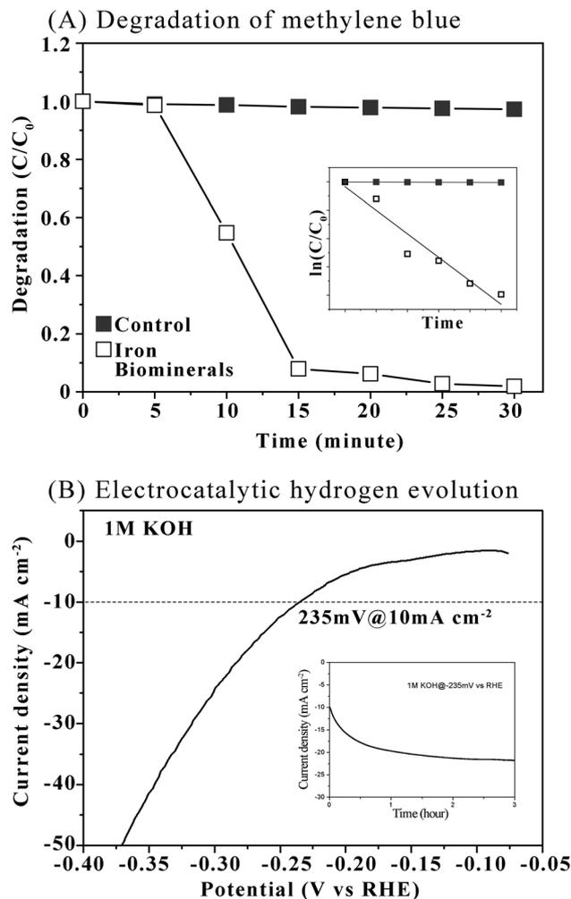
Fig. 7 Panel A shows degradation of methylene blue. Inset of Panel A shows linear relationship between  $\ln(C/C_0)$  and irradiation time. Panel B shows polarization curve of iron biomaterials for HER in 1 M KOH with a potential scan rate of  $5 \text{ mV s}^{-1}$ . Inset of Panel B shows durable operation test of iron biomaterials electrodes operated at designed  $\eta$  ( $10 \text{ mA cm}^{-2}$ ).
