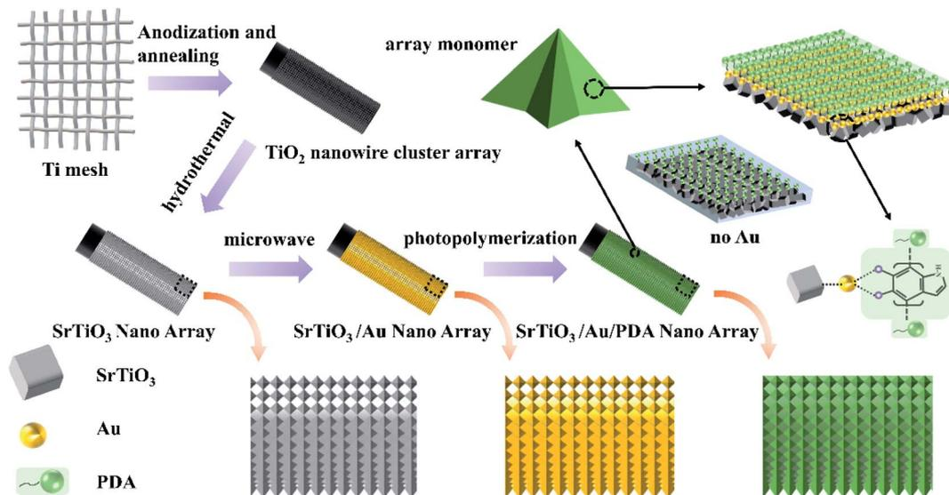
Scheme 1 Process of preparing the 3D hollowed out SrTiO<sub>3</sub>/Au/PDA PEC sensor and schematic of its microscopic appearance.
