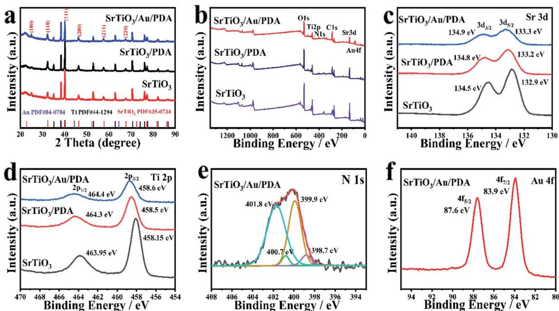
Fig. 2 (a) XRD of SrTiO<sub>3</sub>, SrTiO<sub>3</sub>/PDA, and SrTiO<sub>3</sub>/Au/PDA. (b) Full-range XPS spectra of SrTiO<sub>3</sub>, SrTiO<sub>3</sub>/PDA, and SrTiO<sub>3</sub>/Au/PDA. (c–f) Amplification local XPS of Sr, Ti, N, and Au.
