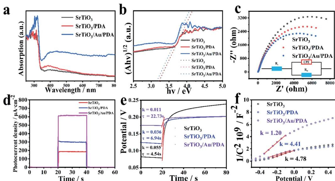
Fig. 3 SrTiO<sub>3</sub>, SrTiO<sub>3</sub>/PDA, and SrTiO<sub>3</sub>/Au/PDA PEC sensors. (a) UV-vis absorption spectra. (b) Plots of  $(Ah\nu)^{1/2}$  and  $h\nu$ . (c) EIS Nyquist plots at 0.4 V vs. Ag/AgCl under light radiation in 0.1 M PBS (pH = 7.4). (d) Photocurrent response. (e) Open-circuit potential plots. (f) Mott-Schottky plots.
