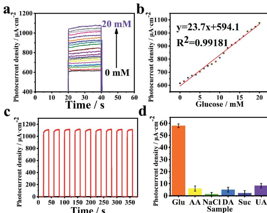
Fig. 4 3D hollowed out SrTiO<sub>3</sub>/Au/PDA/GOx PEC sensor. (a) Photocurrent responses at different glucose concentrations (0–20 mM) in 0.1 M PBS (pH = 7.4). (b) Calibration curve of glucose concentration and photocurrent density. (c) Stability detection curve in 0.1 M PBS (pH = 7.4) at 20 mM of glucose. (d) Histogram of the results of anti-interference analysis (3 mM Glu and 0.3 mM each of AA, NaCl, DA, Suc, and UA).
