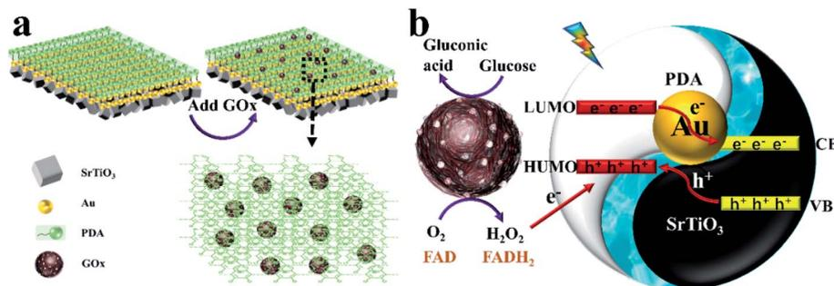
Scheme 2 (a) Modification of GOx on the 3D hollowed out SrTiO<sub>3</sub>/Au/PDA. (b) Mechanism by which gold accelerates photogenerated electron transfer.
