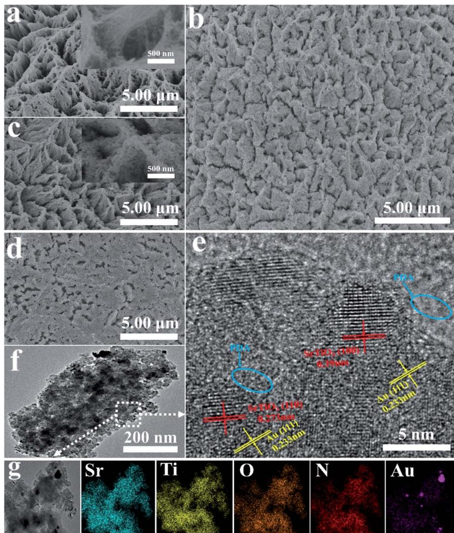
Fig. 1 SEM images of (a)  $\text{TiO}_2$ , (b)  $\text{SrTiO}_3/\text{Au}/\text{PDA}$ , (c)  $\text{SrTiO}_3$ , and (d)  $\text{SrTiO}_3/\text{PDA}$ . (e) HRTEM image of  $\text{SrTiO}_3/\text{Au}/\text{PDA}$ . (f) TEM image of  $\text{SrTiO}_3/\text{Au}/\text{PDA}$ . (g) Mapping of  $\text{SrTiO}_3/\text{Au}/\text{PDA}$  (from left to right: Sr, Ti, O, N, and Au).
