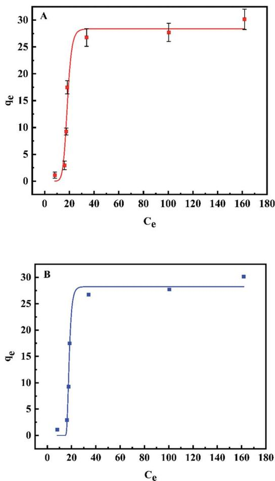
Fig. 9 Fitting plots of the Langmuir adsorption isotherm (A) and Freundlich adsorption isotherm (B). (Temperature: 50 °C, amount of adsorbent: 3 g L<sup>-1</sup>, contact time: 64 min, pH: 4.5).
