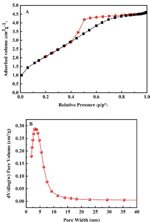
Fig. 4 N<sub>2</sub> adsorption–desorption isotherms (A) and BJH pore size distribution curve (B) of the Al–La hybrid adsorbent.
