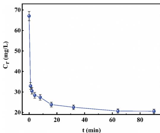
Fig. 7 Effect of contact time (where  $C_r$  ( $\text{mg L}^{-1}$ ) is the residual concentration of fluoride ions, temperature:  $50\text{ }^\circ\text{C}$ , initial fluoride ion concentration:  $70.0\text{ mg L}^{-1}$ , amount of adsorbent:  $3\text{ g L}^{-1}$ , pH: 4.5).
