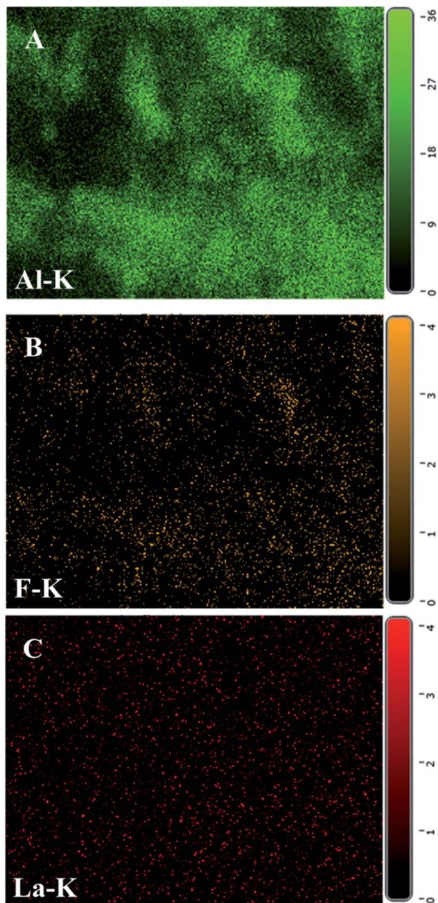
Fig. 12 EDS mapping of Al (A), F (B) and La (C) of the Al-La hybrid adsorbent after adsorption.
