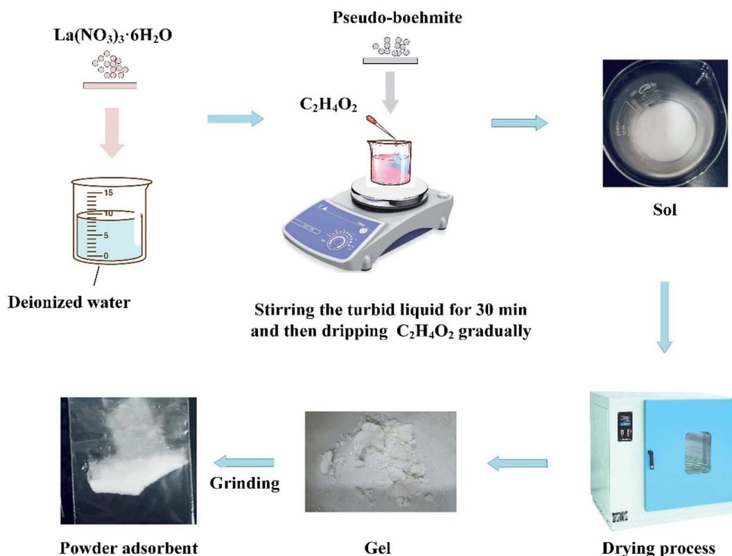
Fig. 1 Schematic diagram of innovative sol–gel method.
