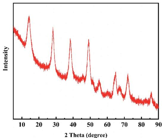
Fig. 2 XRD pattern of the Al-La hybrid adsorbent.
