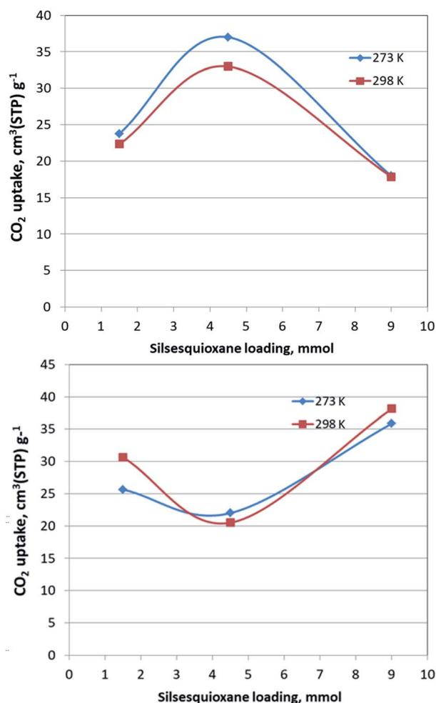
Fig. 8 Gravimetric CO<sub>2</sub> uptake at 1 bar of PILGD<sub>1.5</sub>FD, PILGD<sub>4.5</sub>FD and PILGD<sub>9</sub>FD as a function of silsesquioxane loading at the indicated temperatures (up) and the equivalent measurements for the air-dried samples (down).
