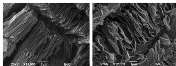
Fig. 7 Representative scanning electron microscopy images of the air-dried (PILGD<sub>4.5</sub>AD, left) and freeze-dried (PILGD<sub>4.5</sub>FD, right) silsesquioxane-pillared GO structures.
