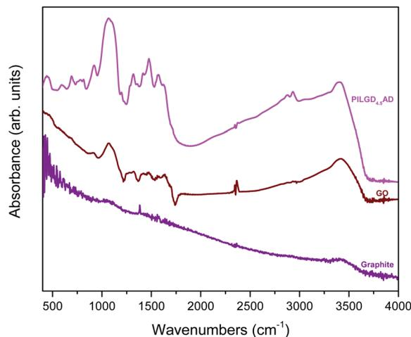
Fig. 5 FTIR spectra of graphite, graphene oxide (GO) and air-dried silsesquioxane-pillared graphene oxide structure PILGD<sub>4.5</sub>AD.
