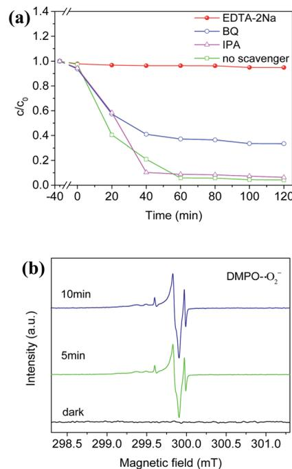
Fig. 6 (a) The photocatalytic activity of RB samples with different quenchers; (b) ESR spectra of DMPO-<sup>•</sup>O<sub>2</sub><sup>-</sup> adducts under light irradiation and in dark.
