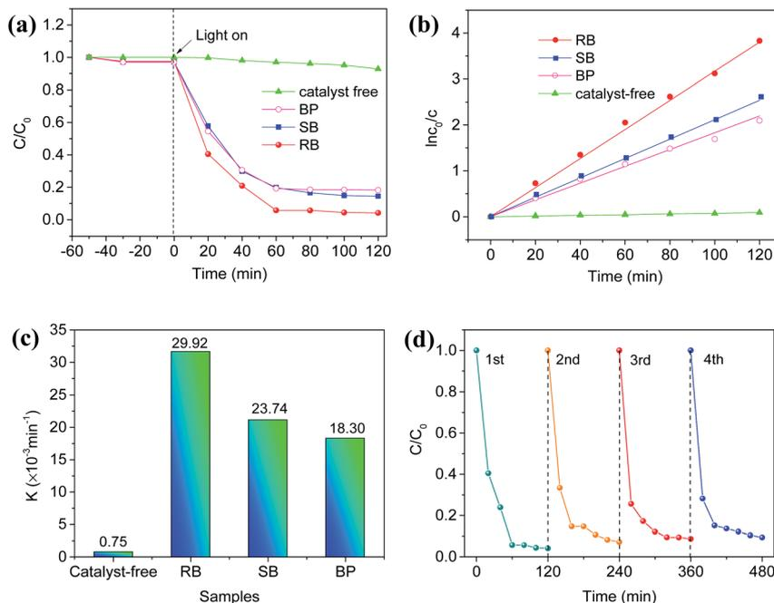
Fig. 5 (a) Photocatalytic degradation of TC over different samples (RB, SB, and BP) in 120 min (the optimum conditions: 50 mg of sample, 20 mg L<sup>-1</sup> of TC solution, pH 9.62, 350 W of the light intensity); (b) the kinetic curves of TC degradation over different samples; (c) the apparent rate constants for TC degradation with different samples; (d) the cyclic degradations of TC over RB samples.
