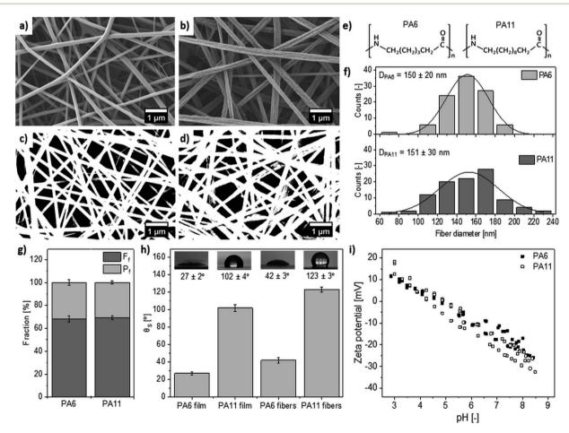
Fig. 1 The SEM images of nanofibers: (a) PA6, (b) PA11. The representative images used in image analysis: (c) PA6, (d) PA11. (e) Structure of repeat units of PA6 and PA11. (f) The histograms of nanofiber diameter distribution. (g) The comparison of fiber  $F_f$  and pore  $P_f$  fractions in the polyamide meshes. (h) Static contact angles for fibers and films. (i) The streaming zeta potential of PA6 and PA11 meshes.
