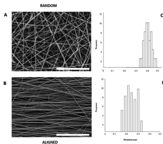
Fig. 2 Morphological analyses of PnNs-loaded electrospun scaffolds: SEM images of (A) random and (B) uni-axial aligned fibres (scale bar 10  $\mu\text{m}$ ); and (C and D) fibre diameter distributions *via* image analysis.
