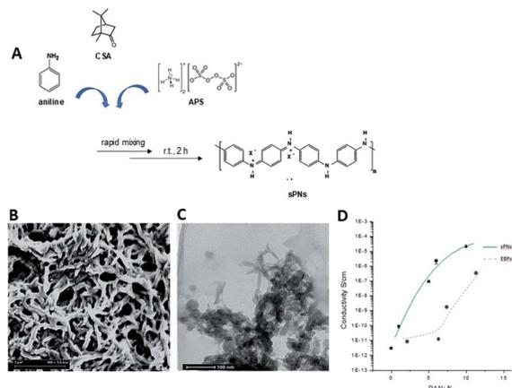
Fig. 1 Optimization of PnNs: (A) scheme of synthesis. Morphological analysis *via* (B) SEM and (C) TEM. Image analysis showed diameters ranging from 50 to 100 nm and lengths from hundreds of nanometers to several micrometers for a nanoneedle shape factor varying from 1 : 9 to 1 : 15. (D) Comparison of conductive curves of PnNs and EBPs obtained by fitting two-probe DC electrical resistance measurements.
