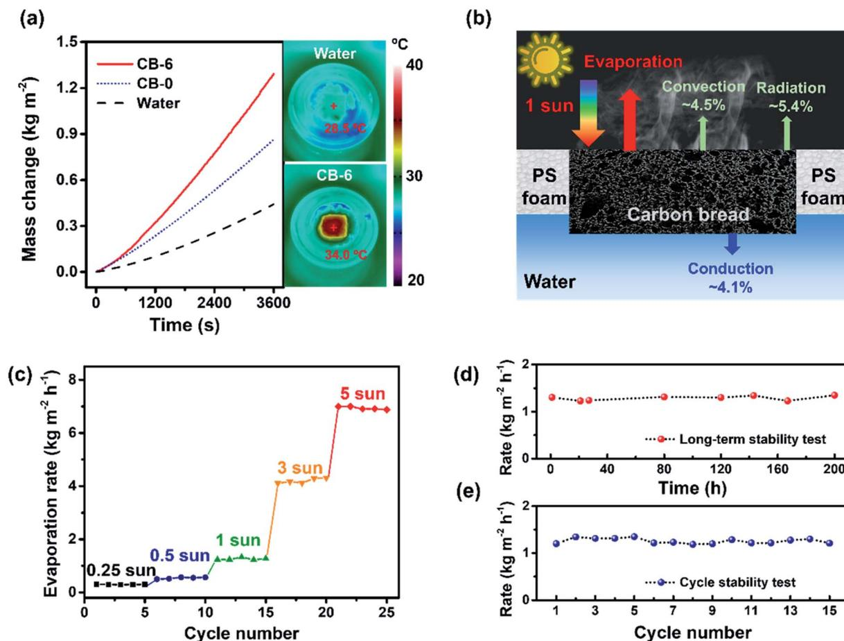
Fig. 5 (a) The left part is the mass change of water with CB-0 and CB-6 under 1 sun solar illumination and the case without CB; the right part shows the IR images under 1 sun with/without CB-6. (b) Diagram of heat transfer in the CB architecture. (c) Water evaporation rate under a series of light intensities. (d) Evaporation rate of CB-6 under 1 sun over 200 hours. (e) Reusability of CB-6 under 1 sun solar illumination for 15 cycles with NaCl solution.
