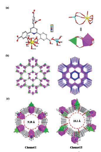
Fig. 1 (a) Structural building block of the  ${\rm TDP^{6-}}$  ligand and  ${\rm [HoZn(CO_2)_6(H_2O)]}$  (C, gray; O, red; Zn, cyan; Ho, yellow; N, blue; and H atoms are omitted for clarity). (b) 3D dual-channel framework of NUC-30 and its topology. (c) View of the 3D channel structure of NUC-30 along the c-axis.
