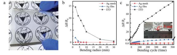
Fig. 3 (a) Optical image of a flexible patterned 8.4 nm Ag film fabricated on a ZnO-coated PE substrate (6 cm  $\times$  6 cm). Relative change in resistance,  $\Delta R/R_0$ , as functions of (b) bending radius and (c) bending cycles at the bending radius of  $\sim$ 5 mm for our 8.4 nm Ag grid TCE (red dots), film TCE (blue triangles), as well as the 180 nm thick ITO (black squares).
