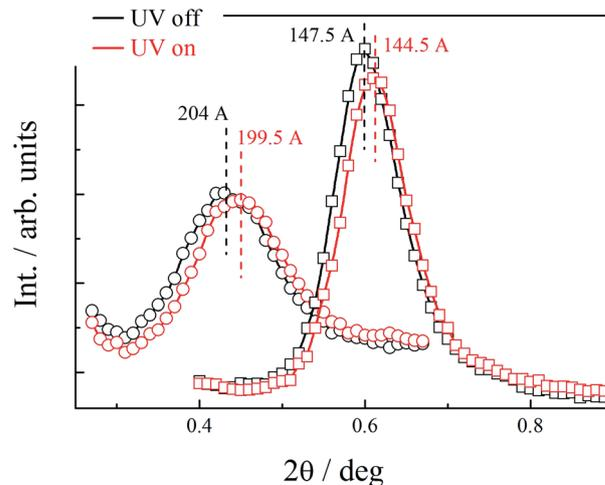
**Fig. 4** Lowest angle XRD signals corresponding to basic periodicity in bilayer (squares) and triple-layer (circles) structures formed by annealed H5 material. Under UV illumination reversible shrinkage of the layers was observed.
