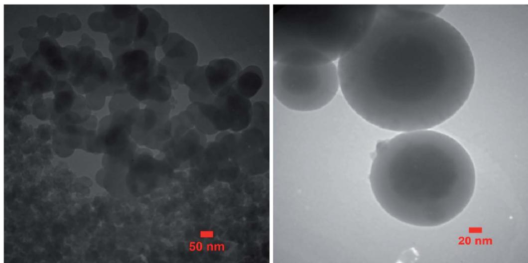
Fig. 6 TEM image of Mo@GAA-Fe<sub>3</sub>O<sub>4</sub> MNPs.
