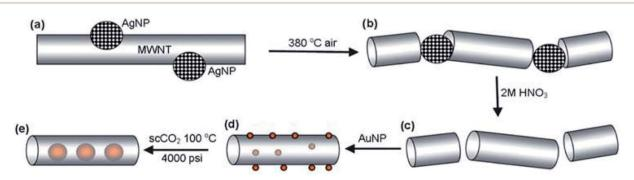
Fig. 3 Scheme showing the proposed mechanism for filling CNTs with Au NPs (a) Ag NPs thiol stabilized on nanotube surface, (b) Ag NPs catalyzed pyrolysis of CNTs, (c) short and open-end nanotubes, (d & e) discrete surface adsorbed Au NPs (red balls) "this figure has been adapted/reproduced from ref. 114 with permission from Royal Society of Chemistry, copyright 2009".
