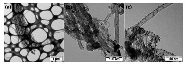
Fig. 5 TEM illustration of VA-CNT functionalized Au NPs "this figure has been adapted/reproduced from ref. 159 with permission from Beilstein Institute for the Advancement of Chemical Sciences, copyright 2014".
