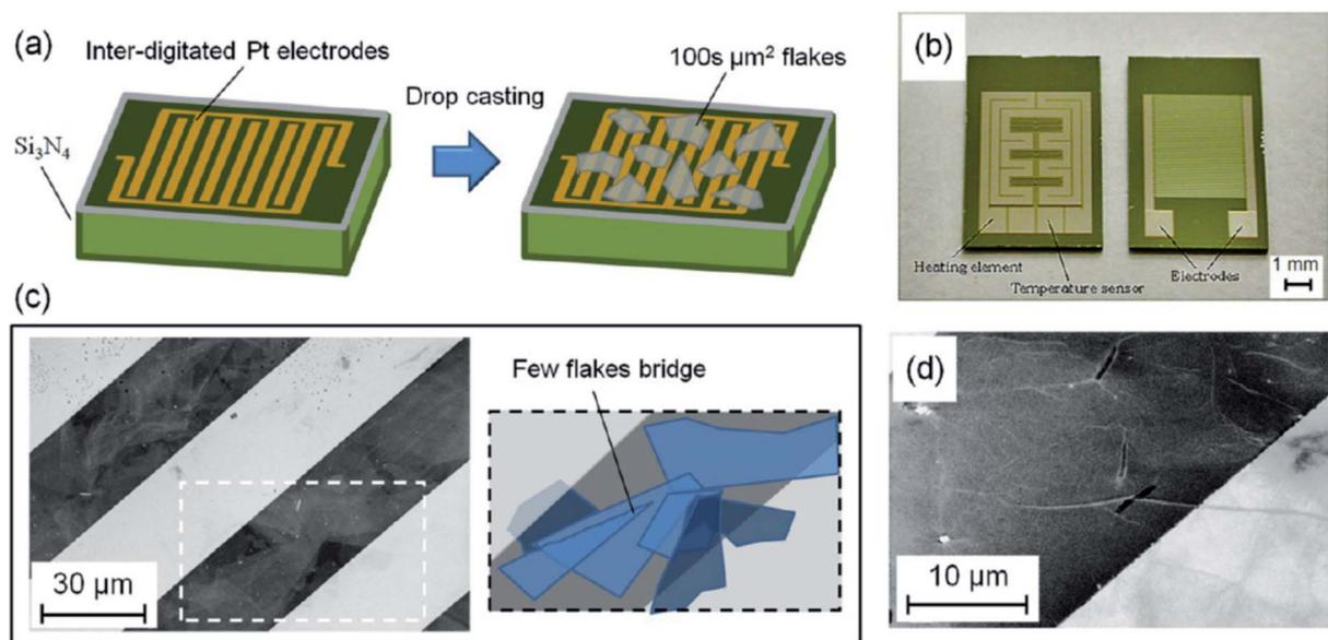
Fig. 2 (a) Schematic depicting the device fabrication, (b) patterned substrate (front-size) with heating elements and temperature sensors on the backside. (c) SEM image of few GO flakes bridging two adjacent Pt electrodes. (d) SEM image of a GO flake lying over an electrode edge. "this figure has been adapted/reproduced from ref. 91 with permission from American Chemical Society, copyright 2013".
