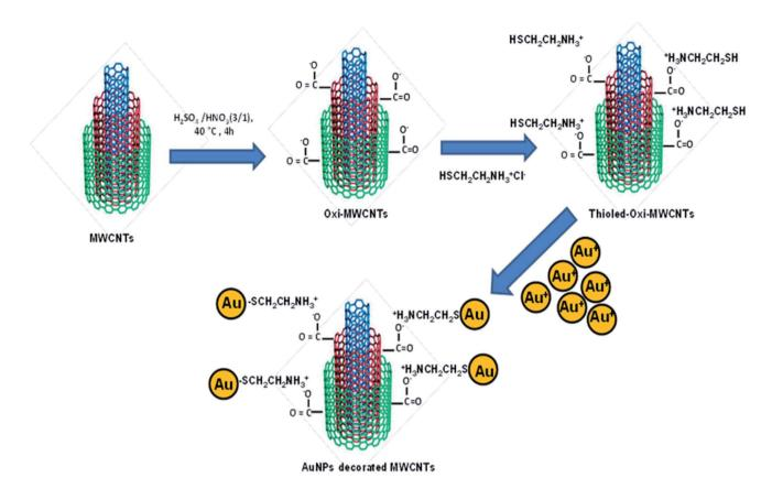
Fig. 4 Schematic illustration of covalent functionalization and decoration of Au NPs on ox-MWCNTs "this figure has been adapted/reproduced from ref. 140 with permission from Springer Nature, copyright 2019".
