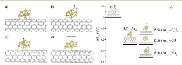
Fig. 11 Ball-and-stick models illustrating (a) (5,5) SWCNTs-Au<sub>13</sub> nanocluster, interactions of adsorbed molecules (b) NO<sub>2</sub>, (c) CO, (d) C<sub>6</sub>H<sub>6</sub>, and (e) theoretical shift of the Fermi energy ( $\Delta E_F$ ) of pristine (5,5) SWCNTs-Au<sub>13</sub>, interaction with C<sub>6</sub>H<sub>6</sub>, CO, and NO<sub>2</sub> gas molecules "this figure has been adapted/reproduced from ref. 168 with permission from American Chemical Society, copyright 2011".
