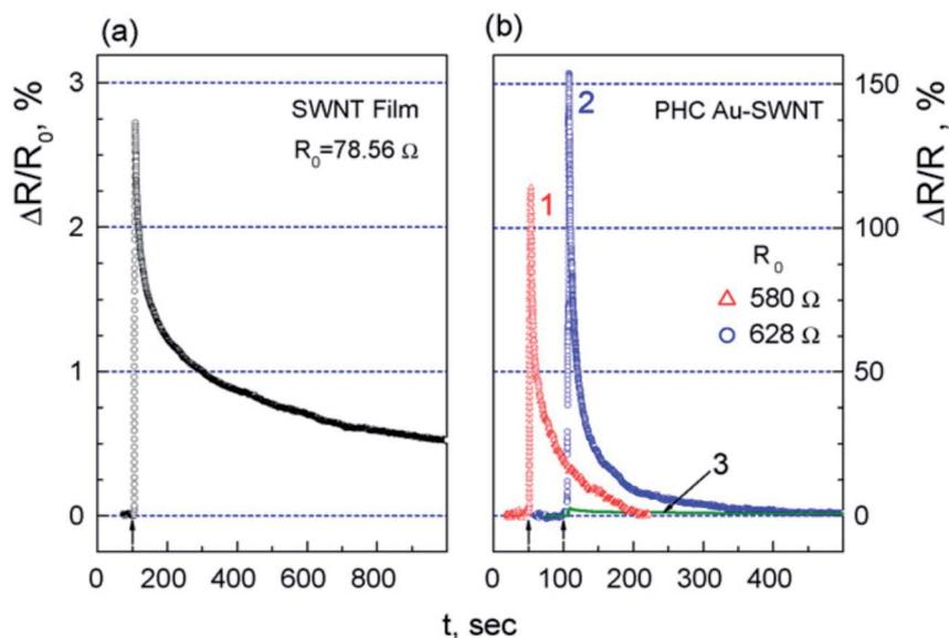
Fig. 9 Change of resistance for (a) SWCNTs film and (b) two Au-SWCNTs heterocontacts in response to 8 s pulse of one percent  $\text{NH}_3$  (curves 1 and 2). For easy comparison with the point contact data on an equal scale, curve 3 represents the data in (a) "this figure has been adapted/reproduced from ref. 192 with permission from Elsevier, copyright 2008".
