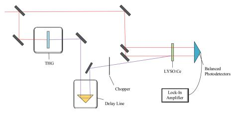
Fig. 2 Schematic diagram of pump-probe experiment settings.
