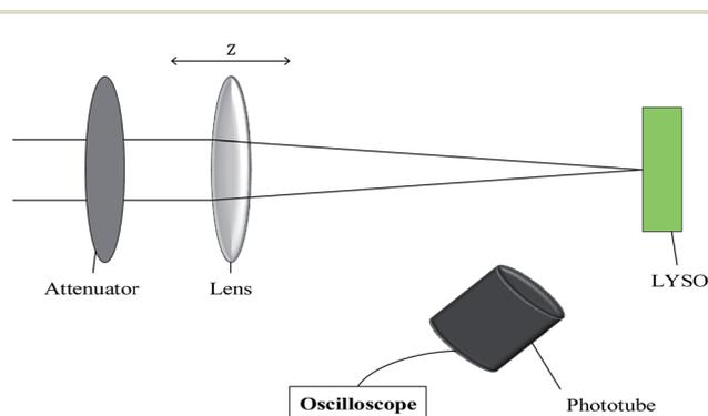
Fig. 1 Schematic diagram of *Z* scan experiment settings.
