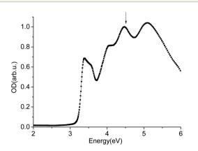
Fig. 9 Absorption spectra of LYSO(Ce).
