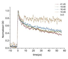
Fig. 8 Normalized OD decay curves of LYSO:Ce excited by different energy laser pulses.
