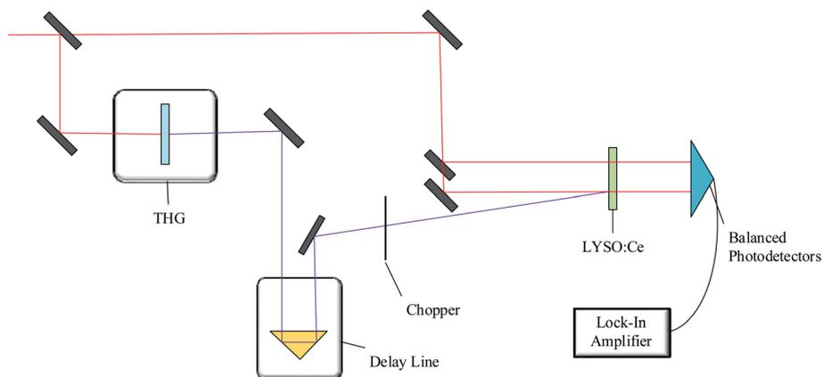
Fig. 2 Schematic diagram of pump-probe experiment settings.
