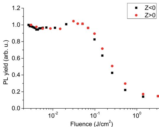
Fig. 5 Normalized PL yield with laser fluence.
