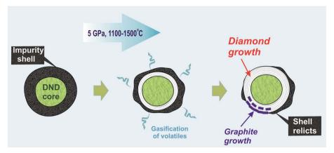
Fig. 6 Schematic drawing of the process of detonation nanodiamond transformation under HPHT annealing. The initial nanodiamond (left grain) at the P-T of the experiment looses a significant part of its shell due to the thermal desorption of the volatiles (grain in the center). The size increase in the nanodiamond core then occurs through the growth of both the diamond phase and ordered graphite (grain to the right).
