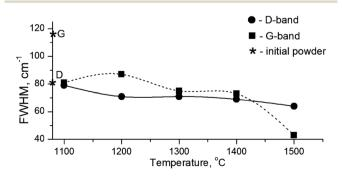
Fig. 5 FWHM values for D- and G-bands in the Raman spectra depending on the annealing temperature. Diamond symbols correspond to the graphite and diamond lines in the initial powder.
