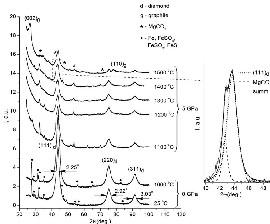
Fig. 1 X-ray diffraction patterns of the initial powder of the detonation nanodiamond, annealed at 0 GPa, and 5 GPa at different temperatures. Inset on the right displays diamond (111) and  $\text{MgCO}_3$  lines in the sample annealed at 1400 °C.
