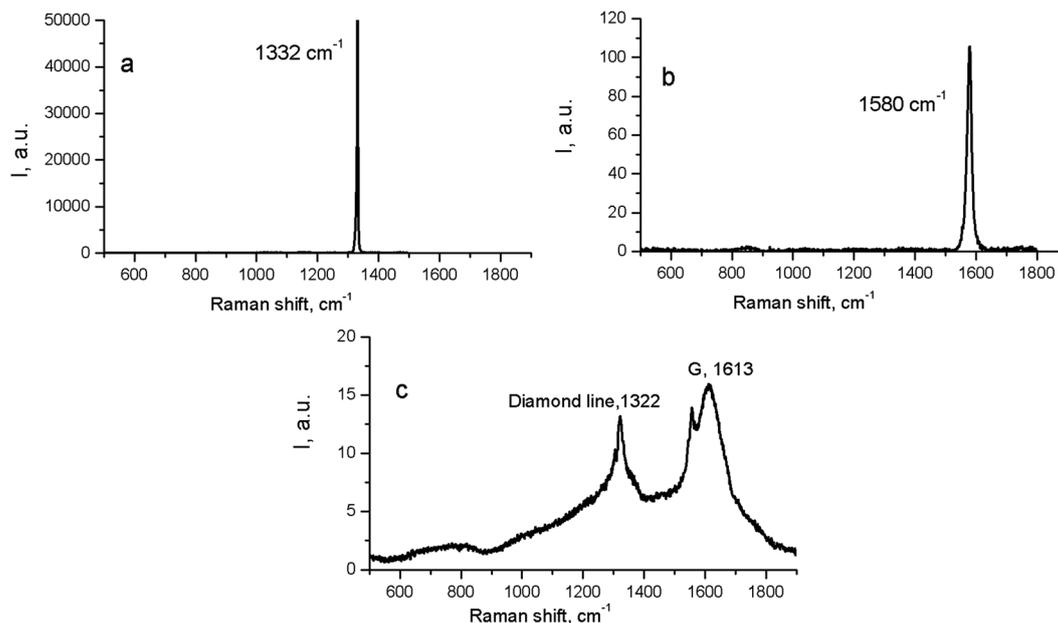
Fig. 3 Raman spectra for natural crystalline cubic diamond (a), graphite (b), and the initial (untreated) detonation nanodiamond (c).
