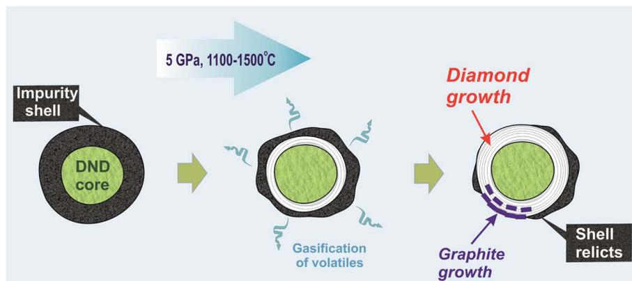
Fig. 6 Schematic drawing of the process of detonation nanodiamond transformation under HPHT annealing. The initial nanodiamond (left grain) at the  $P$ - $T$  of the experiment loses a significant part of its shell due to the thermal desorption of the volatiles (grain in the center). The size increase in the nanodiamond core then occurs through the growth of both the diamond phase and ordered graphite (grain to the right).
