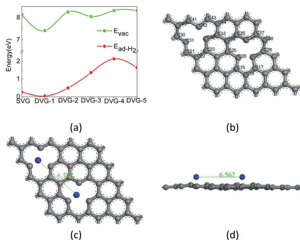
Fig. 2 (a) The adsorption energy and defect formation energy of hydrogen molecules on SVG, DVG-*N* (*N* = 1–5) structures, (b) Adsorption sites, (c) and (d) are the optimized structure of Ti–DVG-4 by molecular dynamic.
