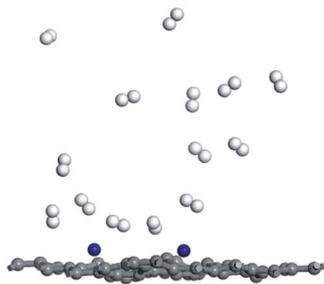
Fig. 5 The hydrogen adsorption geometries of Ti–DVG-4 structure at 400 K.
