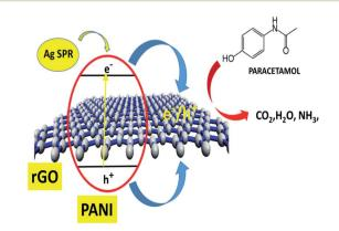
Fig. 10 The plausible degradation mechanism of paracetamol using rGO-Ag/PANI.
