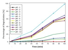
Fig. 5 Effect of pH on the percentage of degradation of paracetamol (25 mg L<sup>-1</sup>) at a fixed amount of rGO-Ag/PANI (50 mg), and room temperature (300 K)
