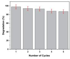
Fig. 11 The recyclability test of rGO-Ag/PANI for the degradation of paracetamol.
