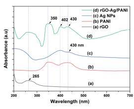
Fig. 1 The UV-Visible absorption spectra of (a) rGO, (b) Ag NPs, (c) PANI, and (d) rGO–Aq/PANI nanocomposites.
