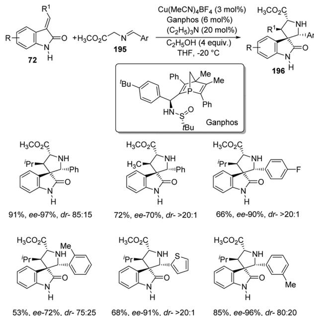
**Scheme 93** Synthesis of spirooxindoles using [Cu(I)/Ganphos] catalytic system.
