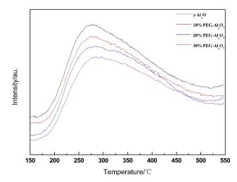
NH<sub>3</sub>-TPD of PEG-modified Al<sub>2</sub>O<sub>3</sub> at different PEG loadings.
