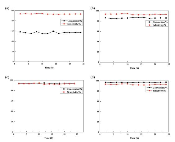
Fig. 5 Catalytic activity of PEG-modified  $Al_2O_3$  at different PEG loadings: (a)  $Al_2O_3$ ; (b) 10% PEG- $Al_2O_3$ ; (c) 20% PEG- $Al_2O_3$ ; and (d) 30% PEG- $Al_2O_3$ .
