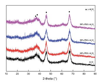
Fig. 1 XRD patterns of PEG-modified Al<sub>2</sub>O<sub>3</sub> at different PEG loadings
