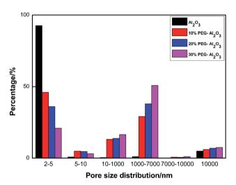
Fig. 2 Pore size distribution of PEG-modified  $Al_2O_3$  at different PEG loadings.
