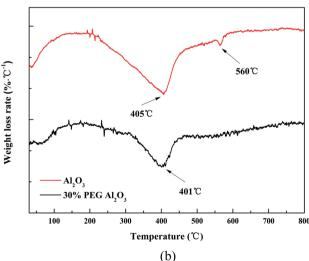
Fig. 3 Characterization of the spent catalysts after the isobutanol dehydration, after 24 hours of reaction. (a) TG-air test, and (b) DTG curves in air.
