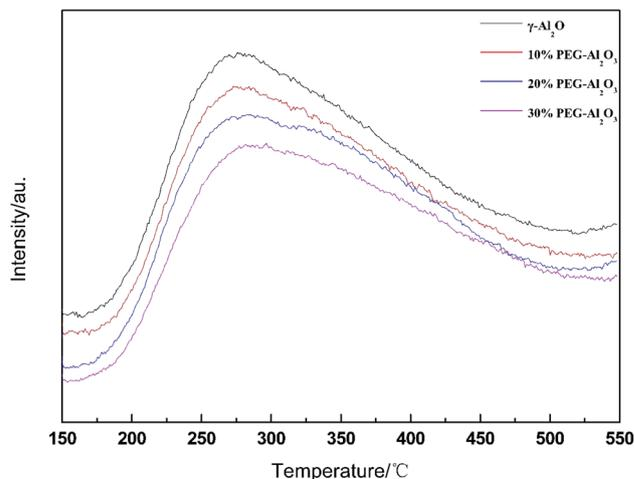
Fig. 4  $\text{NH}_3$ -TPD of PEG-modified  $\text{Al}_2\text{O}_3$  at different PEG loadings.
