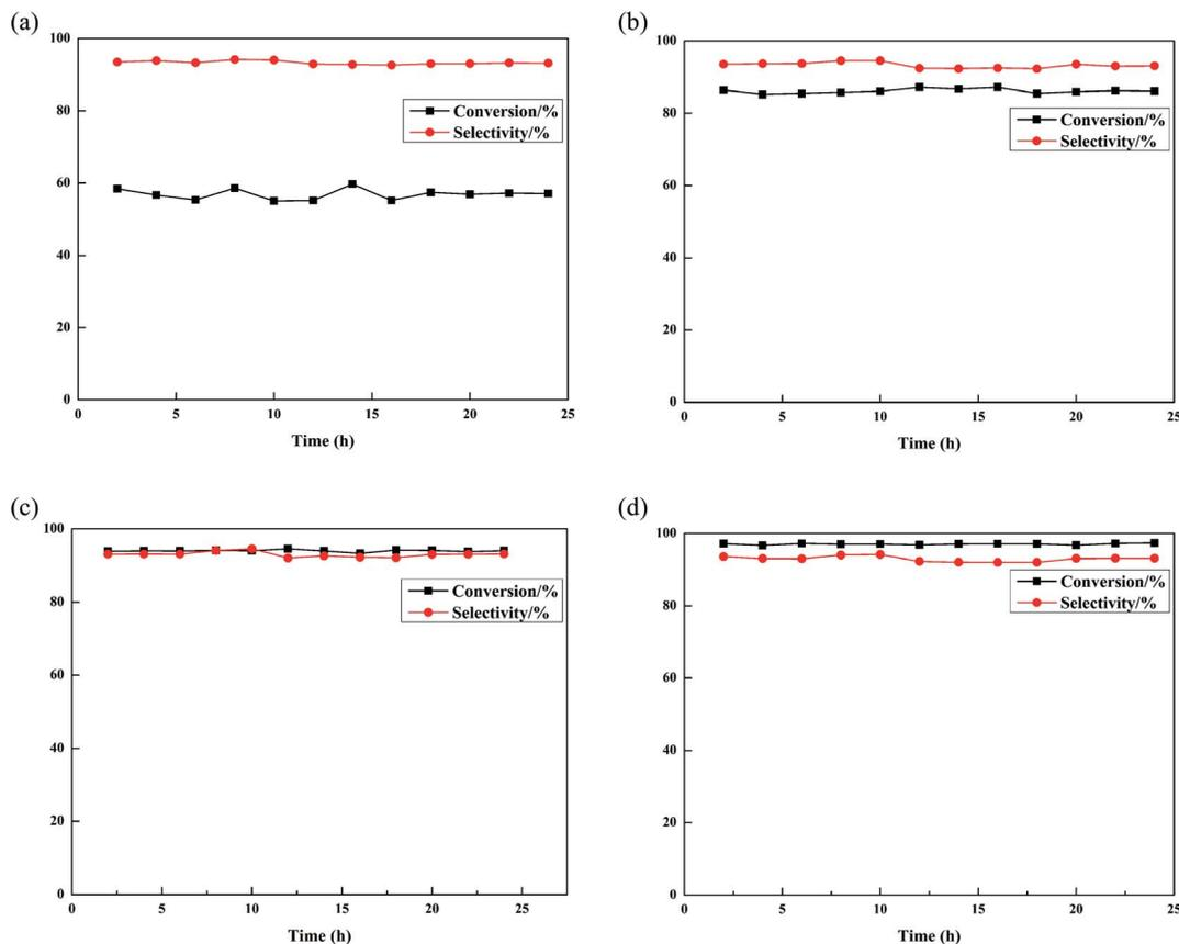
Fig. 5 Catalytic activity of PEG-modified  $\text{Al}_2\text{O}_3$  at different PEG loadings: (a)  $\text{Al}_2\text{O}_3$ ; (b) 10% PEG- $\text{Al}_2\text{O}_3$ ; (c) 20% PEG- $\text{Al}_2\text{O}_3$ ; and (d) 30% PEG- $\text{Al}_2\text{O}_3$ .
