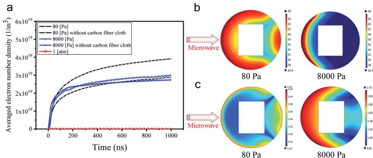
Fig. 6 (a) Variation of the averaged electron number density with time; (b) natural logarithm distribution of the electron number density ( $\ln(n_e)$ ) at the time of 1000 ns ( $n_e$  is in the unit of  $m^{-3}$ ); (c) distributions of electron temperature at the time of 1000 ns (unit: eV).
