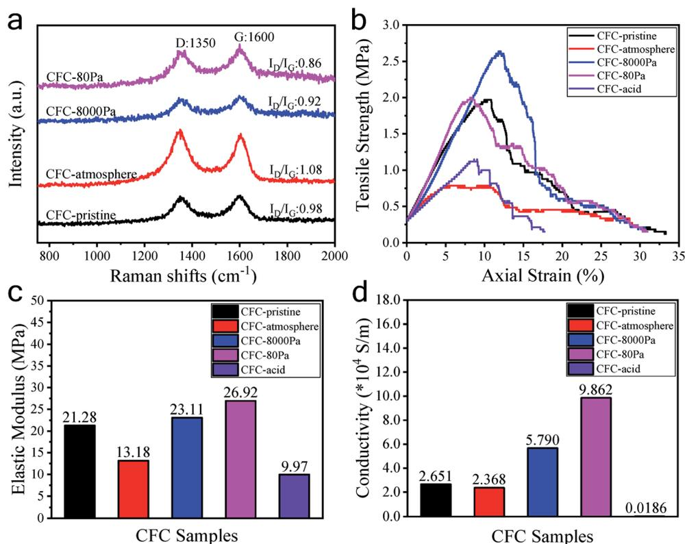
Fig. 4 Raman spectra (a), tensile strength values (b), elastic modulus values (c), and conductivity values (d) of the CFC samples.
