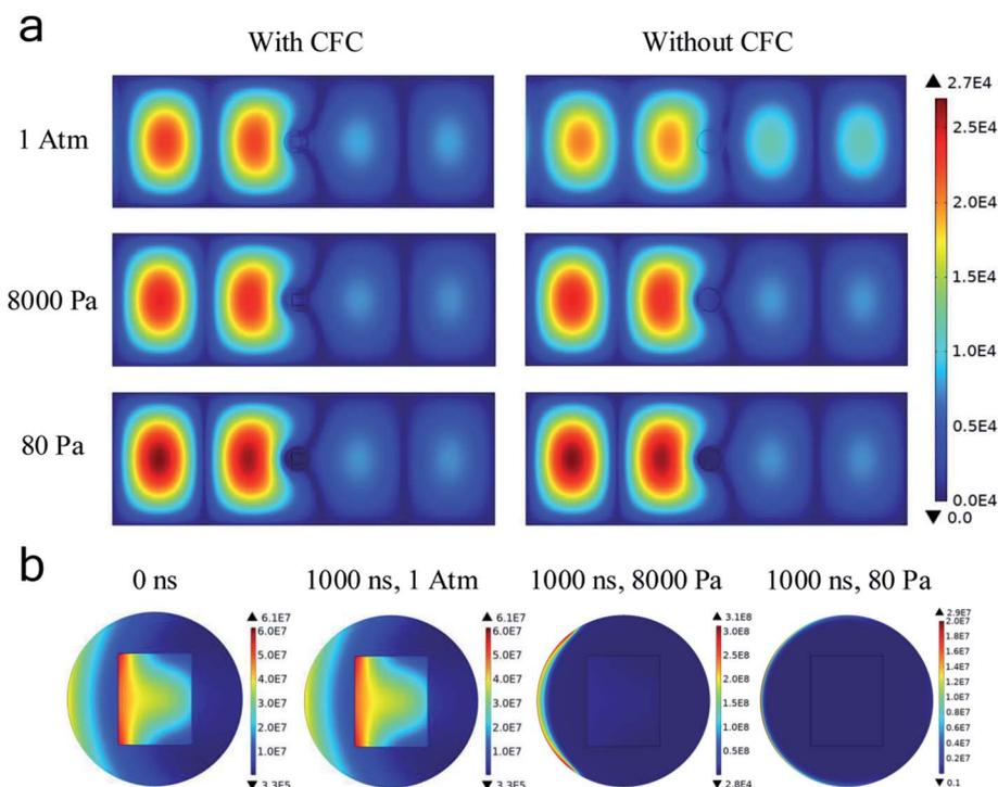
Fig. 5 (a) Distributions of the microwave electric field under different reacting conditions at the time of 1000 ns (unit: V m<sup>-1</sup>); (b) distribution of microwave power dissipation at all pressures with CFC (unit: W m<sup>-3</sup>).
