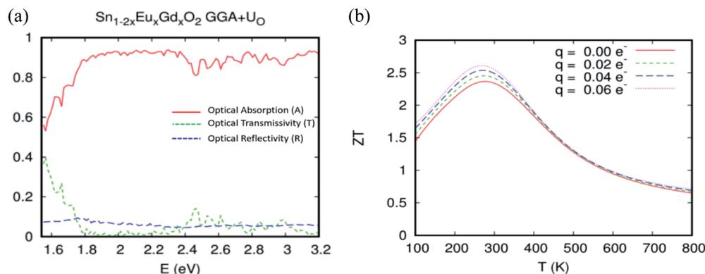
Fig. 11 The GGA+U calculation for  $\text{Sn}_{0.9375}\text{Eu}_{0.0625}\text{Gd}_{0.0625}\text{O}_2$  with the Hubbard coefficient applied only for the anion p states of the host system for a Eu–Gd separation of 3.24 Å. (a) Optical absorption, transmissivity, and reflectivity. (b) Figure of merit ( $zT$ ), as a function of doping for different temperatures.
