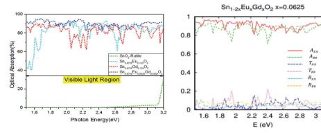
Fig. 9 The (a) optical absorption in visible light for  $SnO_2$ ,  $Sn_{0.875}Eu_{0.125}O_2$ ,  $Sn_{0.875}Gd_{0.125}O_2$ , and  $Sn_{0.125}Eu_{0.0625}Gd_{0.0625}O_2$ , with a fixed slab thickness of d=1000 nm. (b) Optical absorption, transmissivity, and reflectivity in different crystallographic directions for  $Sn_{0.9375}Eu_{0.0625}Gd_{0.0625}O_2$ , with a fixed slab thickness of d=1000 nm.
