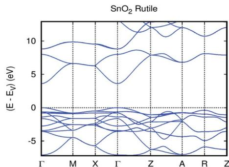
Fig. 2 The GGA+U band structure of SnO<sub>2</sub> rutile.
