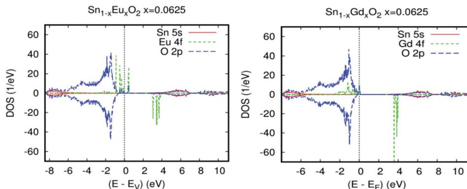
Fig. 3 (a) Projected local DOS for Sn<sub>0.9375</sub>Eu<sub>0.0625</sub>O<sub>2</sub>, (b) Projected local DOS for Sn<sub>0.9375</sub>Gd<sub>0.0625</sub>O<sub>2</sub>. Fermi level is set at zero.
