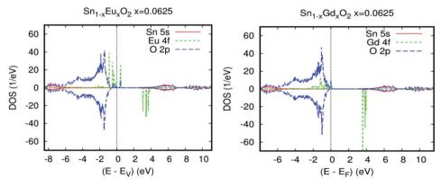
Fig. 3 (a) Projected local DOS for Sn<sub>0.9375</sub>Eu<sub>0.0625</sub>O<sub>2</sub>, (b) Projected local DOS for Sn<sub>0.9375</sub>Gd<sub>0.0625</sub>O<sub>2</sub>. Fermi level is set at zero.
