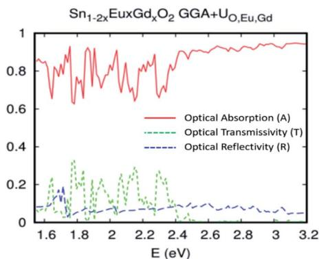
Fig. 12 The GGA+U calculation for optical absorption, transmissivity, and reflectivity of  $\text{Sn}_{0.9375}\text{Eu}_{0.0625}\text{Gd}_{0.0625}\text{O}_2$ , for a Eu–Gd separation of 3.24 Å. The Hubbard coefficient is simultaneously applied to the anion p states and 4f electrons.
