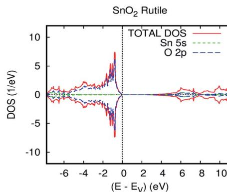
Fig. 1 The GGA total and partial DOS of SnO<sub>2</sub> rutile.
