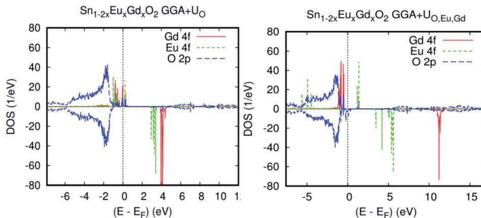
Fig. 6 The GGA+U PLDOSs of  $\text{Sn}_{1-2x}\text{Eu}_x\text{Gd}_x\text{O}_2$  for an Eu–Gd separation of 3.24 Å. (a) The Hubbard coefficient was applied only to the anion p states of a host system. (b) The Hubbard coefficient was simultaneously applied to the anion p states and 4f electrons.
