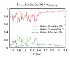
Fig. 12 The GGA+U calculation for optical absorption, transmissivity, and reflectivity of  $Sn_{0.9375}Eu_{0.0625}Gd_{0.0625}O_2$ , for a Eu-Gd separation of 3.24 Å. The Hubbard coefficient is simultaneously applied to the anion p states and 4f electrons.
