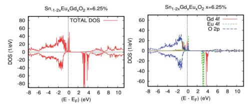
Fig. 5 Calculated spin-resolved density of states (DOS) for  $Sn_{0.9375}Eu_{0.0625}Gd_{0.0625}O_2$ , for an Eu-Gd separation of 3.24 Å. (a) The total DOS, and (b) the partial DOS of neighbouring Sn-5s, O-2p, and RE-4f states. The Fermi level is set at zero.
