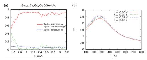
Fig. 11 The GGA+U calculation for  $Sn_{0.9375}Eu_{0.0625}Gd_{0.0625}$   $O_2$  with the Hubbard coefficient applied only for the anion p states of the host system for a Eu-Gd separation of 3.24 Å. (a) Optical absorption, transmissivity, and reflectivity. (b) Figure of merit (ZT), as a function of doping for different temperatures.
