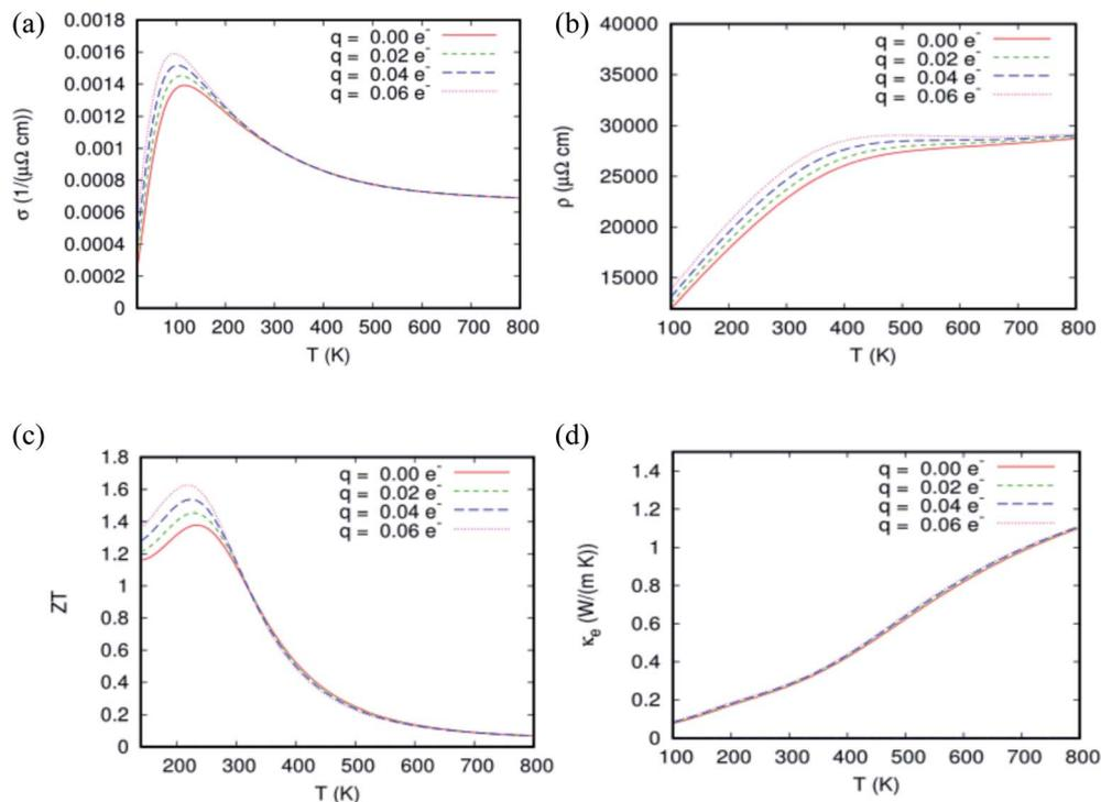
Fig. 10 (a–d) A plot of transport properties for  $\text{Sn}_{0.875}\text{Eu}_{0.065}\text{Gd}_{0.065}\text{O}_2$  as a function of doping for different temperatures. (a) Electrical conductivity, (b) electrical resistivity, (c) figure of merit ( $zT$ ), and (d) thermal electrical conductivity.
