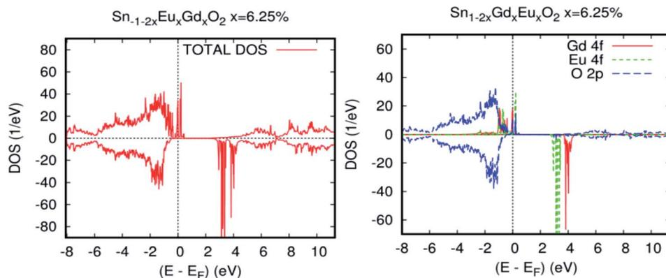
Fig. 5 Calculated spin-resolved density of states (DOS) for  $\text{Sn}_{0.9375}\text{Eu}_{0.0625}\text{Gd}_{0.0625}\text{O}_2$ , for an Eu–Gd separation of 3.24 Å. (a) The total DOS, and (b) the partial DOS of neighbouring Sn-5s, O-2p, and RE-4f states. The Fermi level is set at zero.
