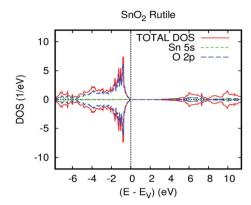
Fig. 1 The GGA total and partial DOS of SnO<sub>2</sub> rutile.
