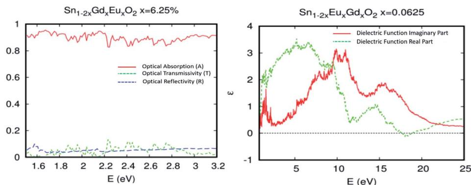
Fig. 8 (a) The optical absorption, transmissivity, and reflectivity in visible light for  $\text{Sn}_{1-2x}\text{Gd}_x\text{Eu}_x\text{O}_2$   $x = 0.0625$ , with a fixed slab thickness of  $d = 1000$  nm. (b) The real and imaginary part of the dielectric function *versus* energy for  $\text{Sn}_{1-2x}\text{Gd}_x\text{Eu}_x\text{O}_2$   $x = 0.0625$ .
