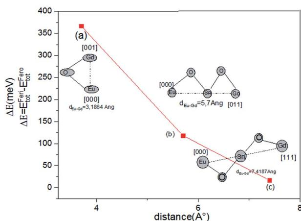
**Fig. 4** The energy difference between ferromagnetic and ferrimagnetic configurations vs. Eu–Gd distance in the unit cell for  $\text{Sn}_{0.875}\text{Eu}_{0.065}\text{Gd}_{0.065}\text{O}_2$ .
