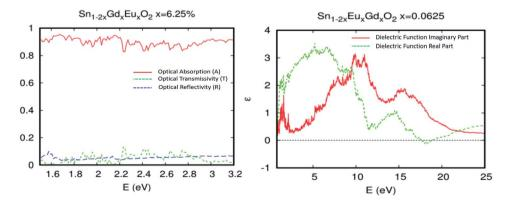
Fig. 8 (a) The optical absorption, transmissivity, and reflectivity in visible light for  $Sn_{1-2x}Gd_xEu_xO_2$  x=0.0625, with a fixed slab thickness of d=0.0625, where d=0.0625, where d=0.0625 is the optical absorption of the optical absorpti 1000 nm. (b) The real and imaginary part of the dielectric function versus energy for  $Sn_{1-2x}Gd_xEu_xO_2$  x=0.0625.
