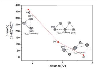
Fig. 4 The energy difference between ferromagnetic and ferrimagnetic configurations vs. Eu–Gd distance in the unit cell for  $Sn_{0.875}Eu_{0.065}Gd_{0.065}O_2$ .
