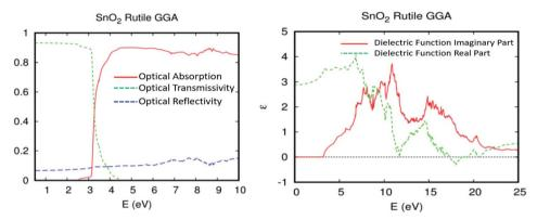
Fig. 7 (a) The optical absorption, transmissivity, and reflectivity, and (b) the real and imaginary parts of the dielectric function for SnO<sub>2</sub> rutile.
